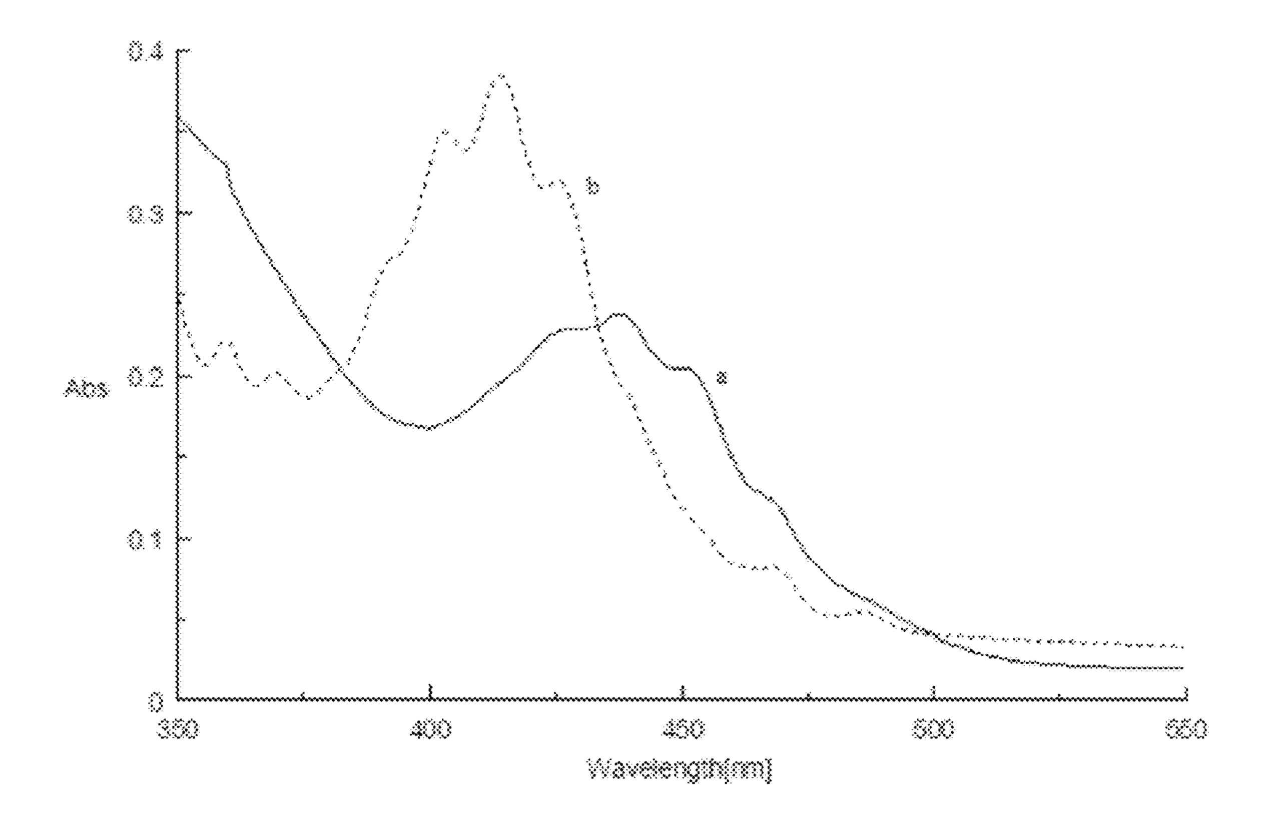
(a) 80% uranyl nitrate-titania sol; (b) uranyl nitrate solution in water
