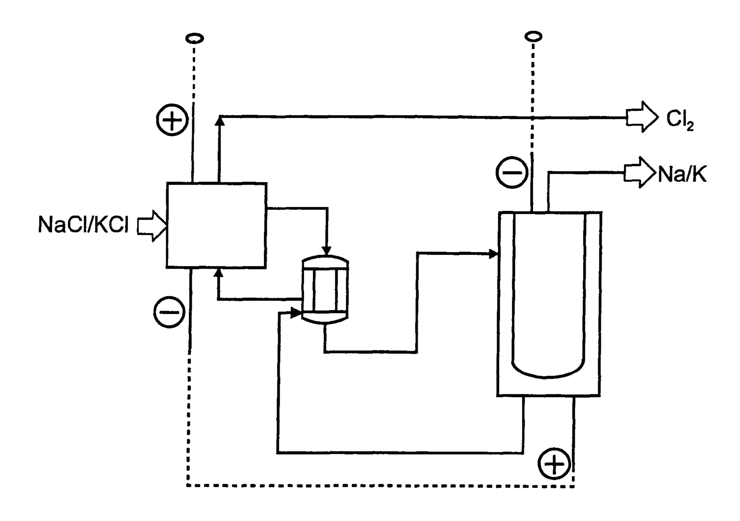
SOLID POLYCRYSTALLINE POTASSIUM ION CONDUCTOR HAVING A β"-AL<sub>2</sub>O<sub>3</sub> STRUCTURE, ITS PRODUCTION AND THE PREPARATION OF POTASSIUM METAL USING THIS POTASSIUM ION CONDUCTOR
