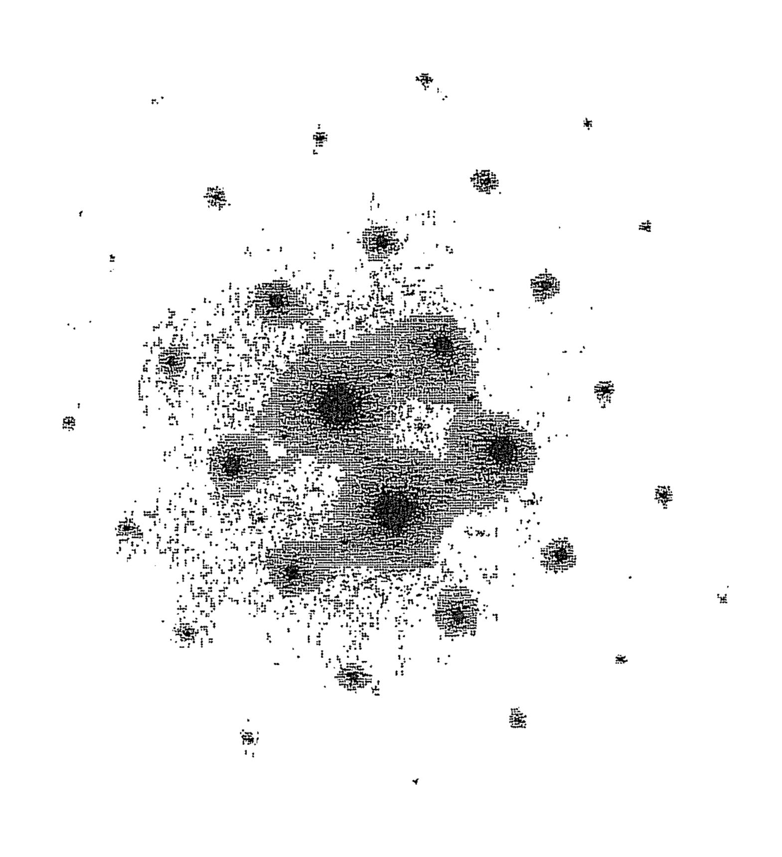
FIG. 1. Selected area diffraction pattern of Alloy #1 (heat treatment B) obtained using transmission electron microscopy (TEM) instrument, showing matrix and  $\gamma'$  diffracted spots.
