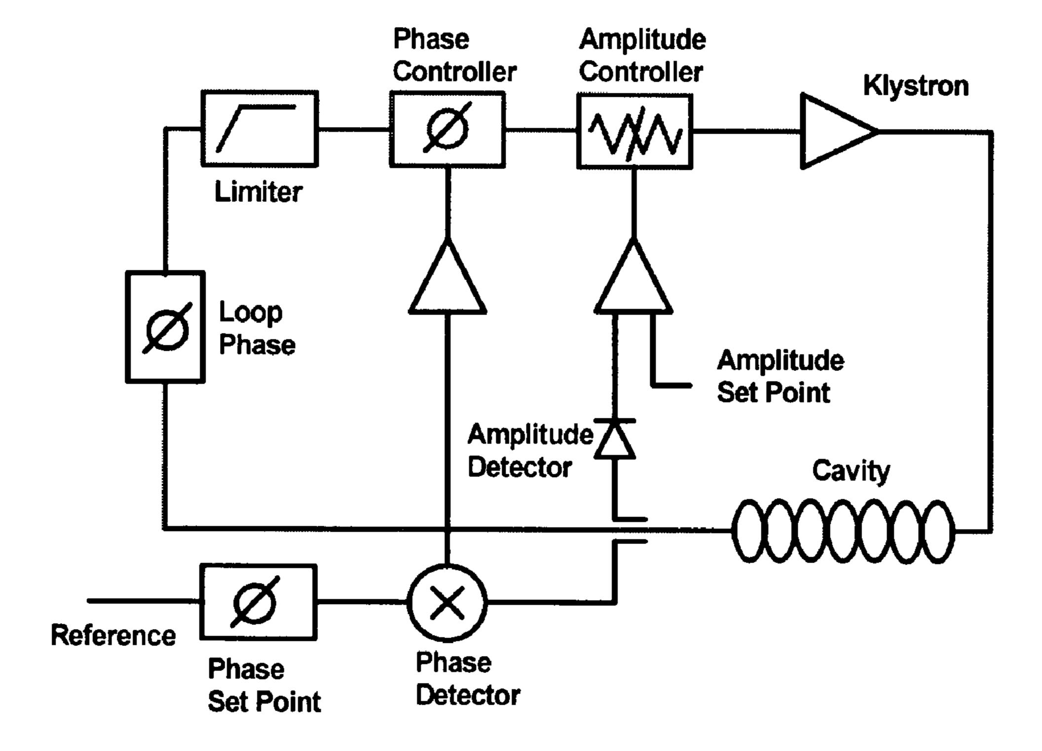
Figure 1: SEL Block Diagram
