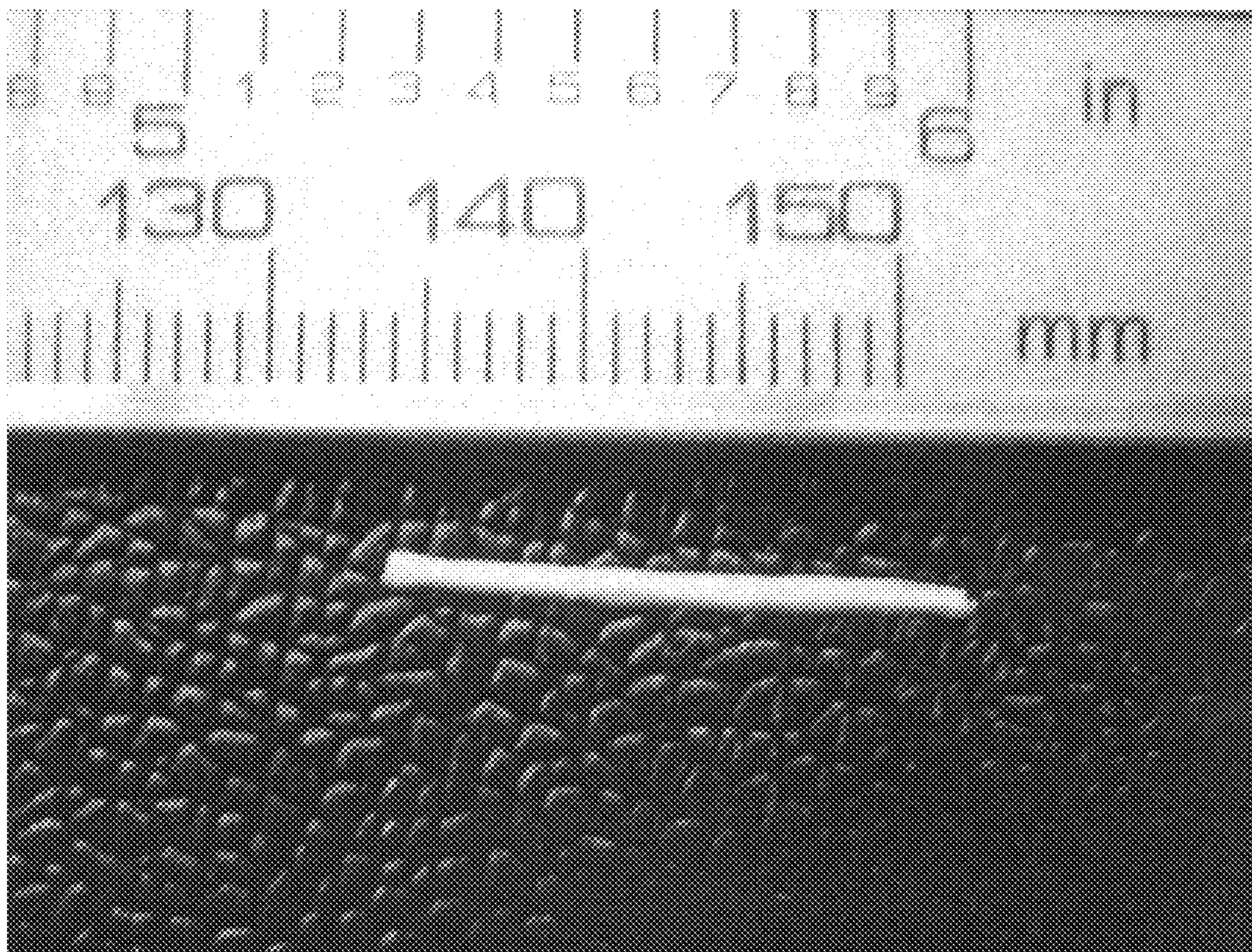
Figure 12b. Drug eluting nerve guide tube after removal from mandrel.
