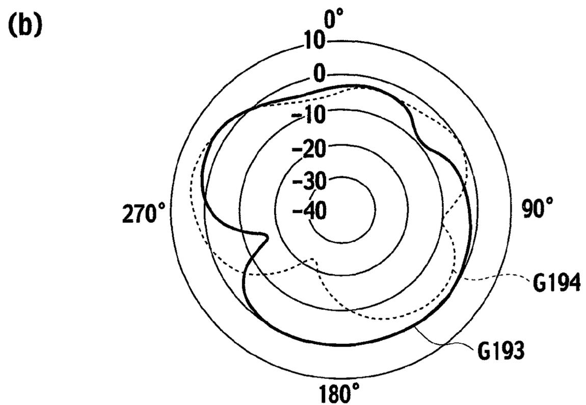
RADIATION CHARACTERISTIC OF xy PLANE (S=0 ; Unit:dBi)
