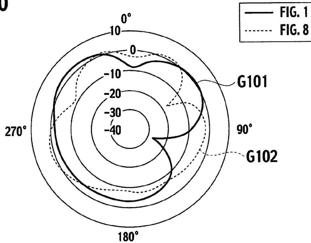
RADIATION CHARACTERISTIC (xy PLANE Unit:dBi)
