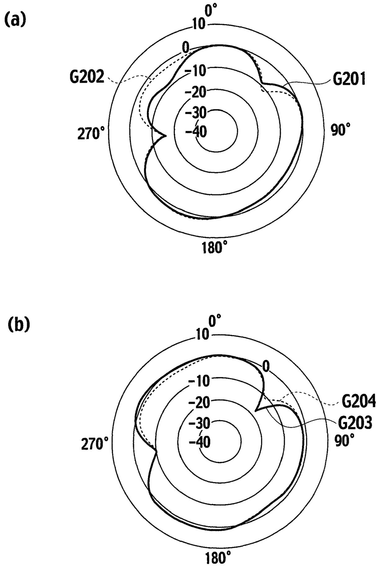
RADIATION CHARACTERISTIC OF xy PLANE (S=16 ; Unit:dBi)
