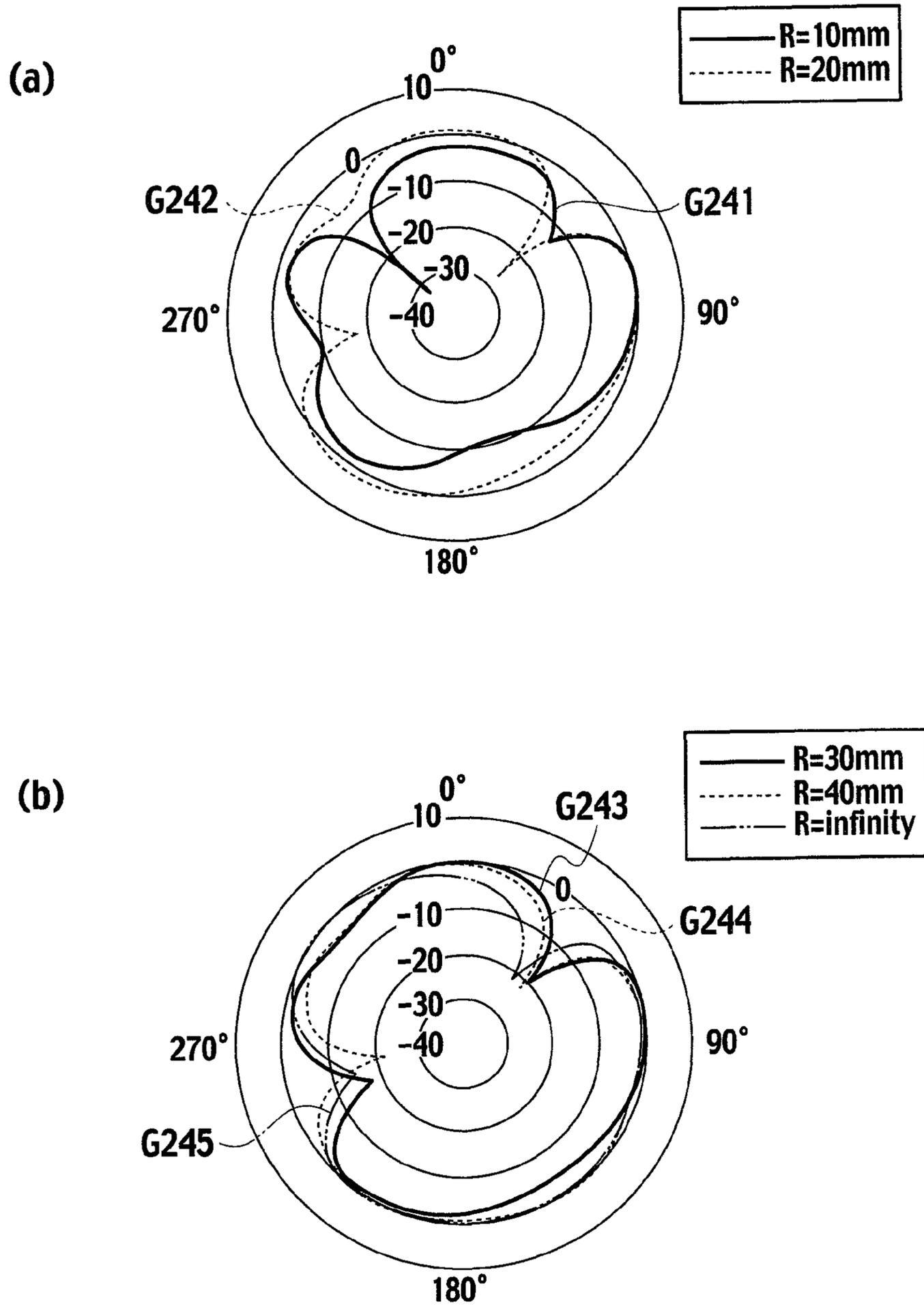
RADIATION CHARACTERISTIC OF xy PLANE (Unit:dBi)
