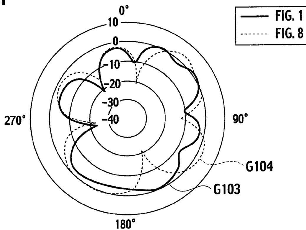
RADIATION CHARACTERISTIC (yz PLANE Unit:dBi)
