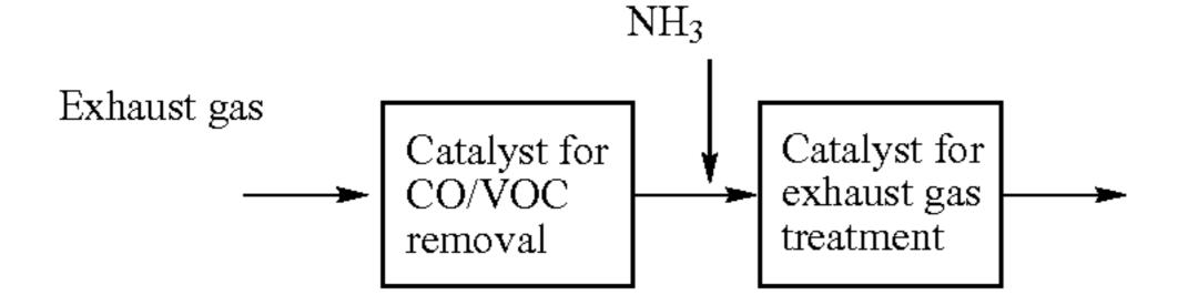
Tables 3 and 5 to 9 demonstrated that Examples 3 to 8 wherein the zone of the exhaust gas treating catalyst was placed upstream the zone of the CO/VOC removal catalyst improved the total reaction rate of CO at all the temperatures from 200 to 400° C., as compared with Comparative Examples 2 and 3 wherein the zone of the exhaust gas treating catalyst was placed downstream the zone of the CO/VOC removal catalyst.
