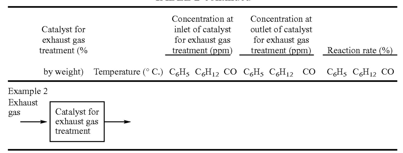
Tables 1 and 2 demonstrated that the VOCs of various kinds <sup>15</sup> are partially oxidized to CO in the zone of the exhaust gas treating catalyst in Examples 1 to 2.
