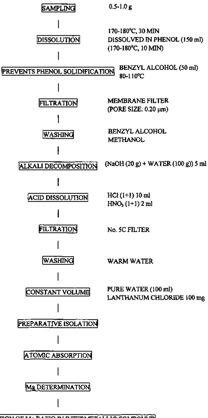
DETERMINATION OF Mg RATIO IN INTERMETALLIC COMPOUND
