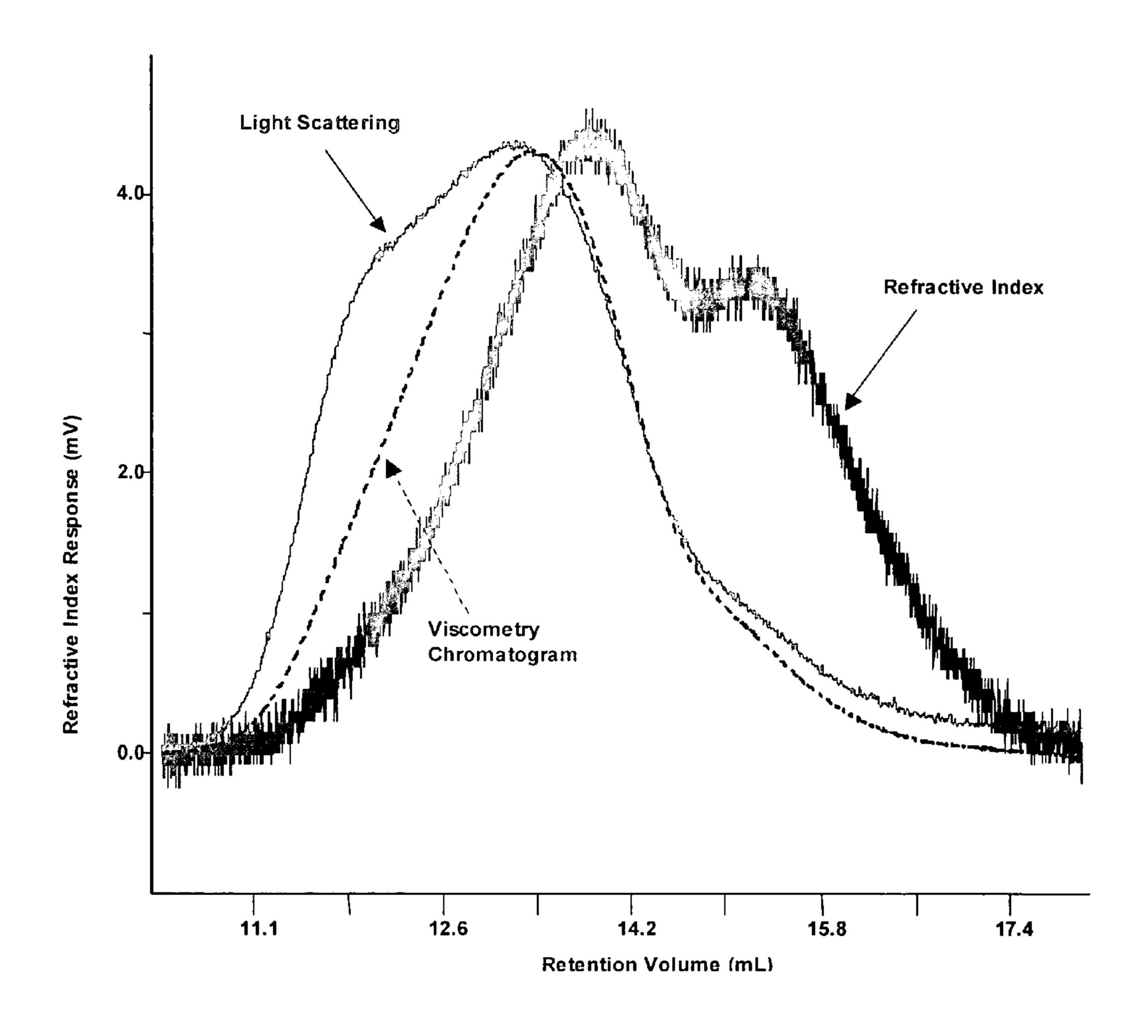
Figure 2. Typical chromatograms of CMC with Glycerin using aqueous SEC with triple detection (Formulation-8)
