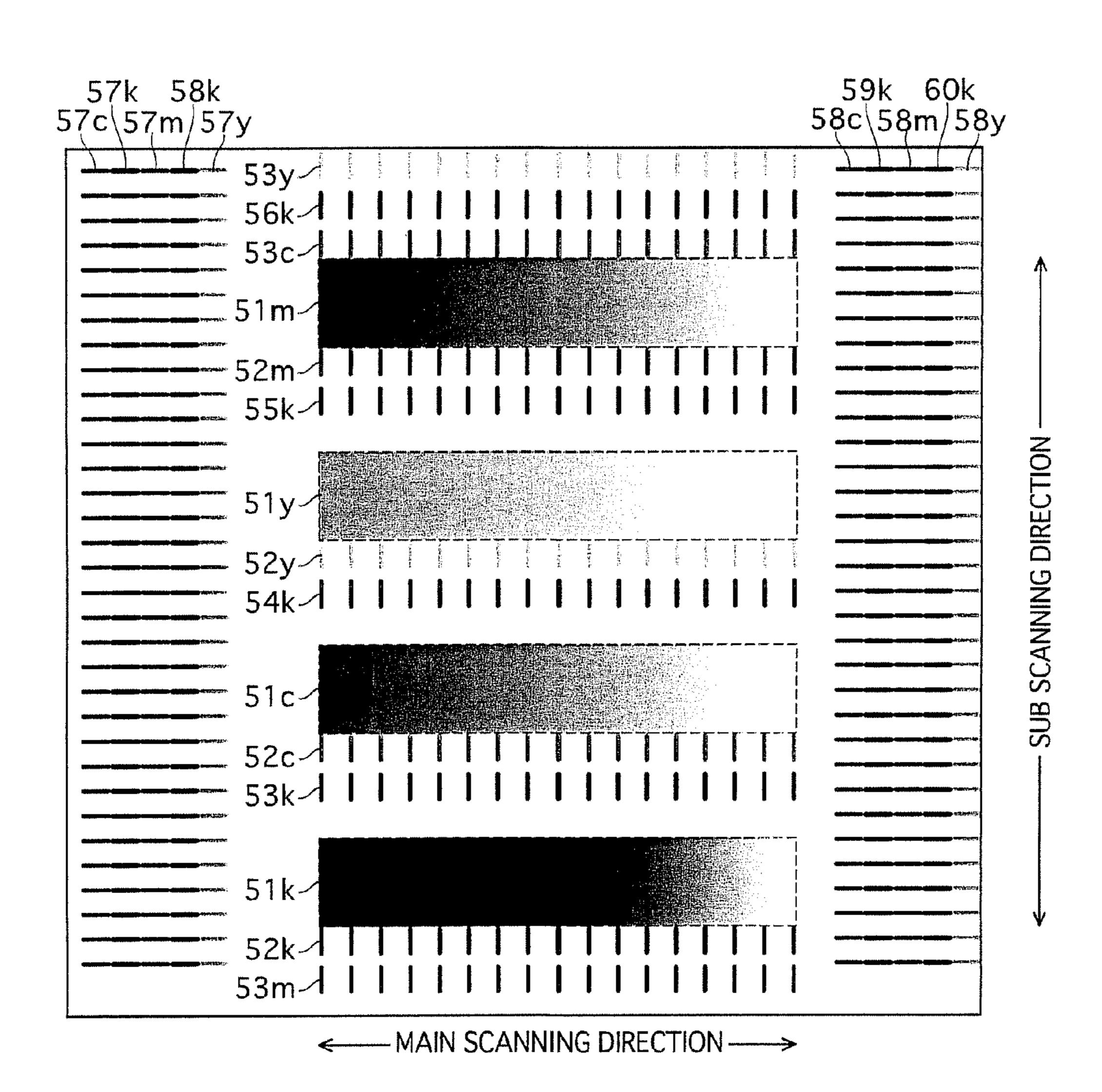
IMAGE FORMING APPARATUS, TONE CORRECTION METHOD USING TONE PATCHES AND ALIGNMENT MARKERS, AND COMPUTER-READABLE RECORDING MEDIUM RECORDED WITH A TONE **CORRECTION PROGRAM USING TONE** PATCHES AND ALIGNMENT MARKERS
