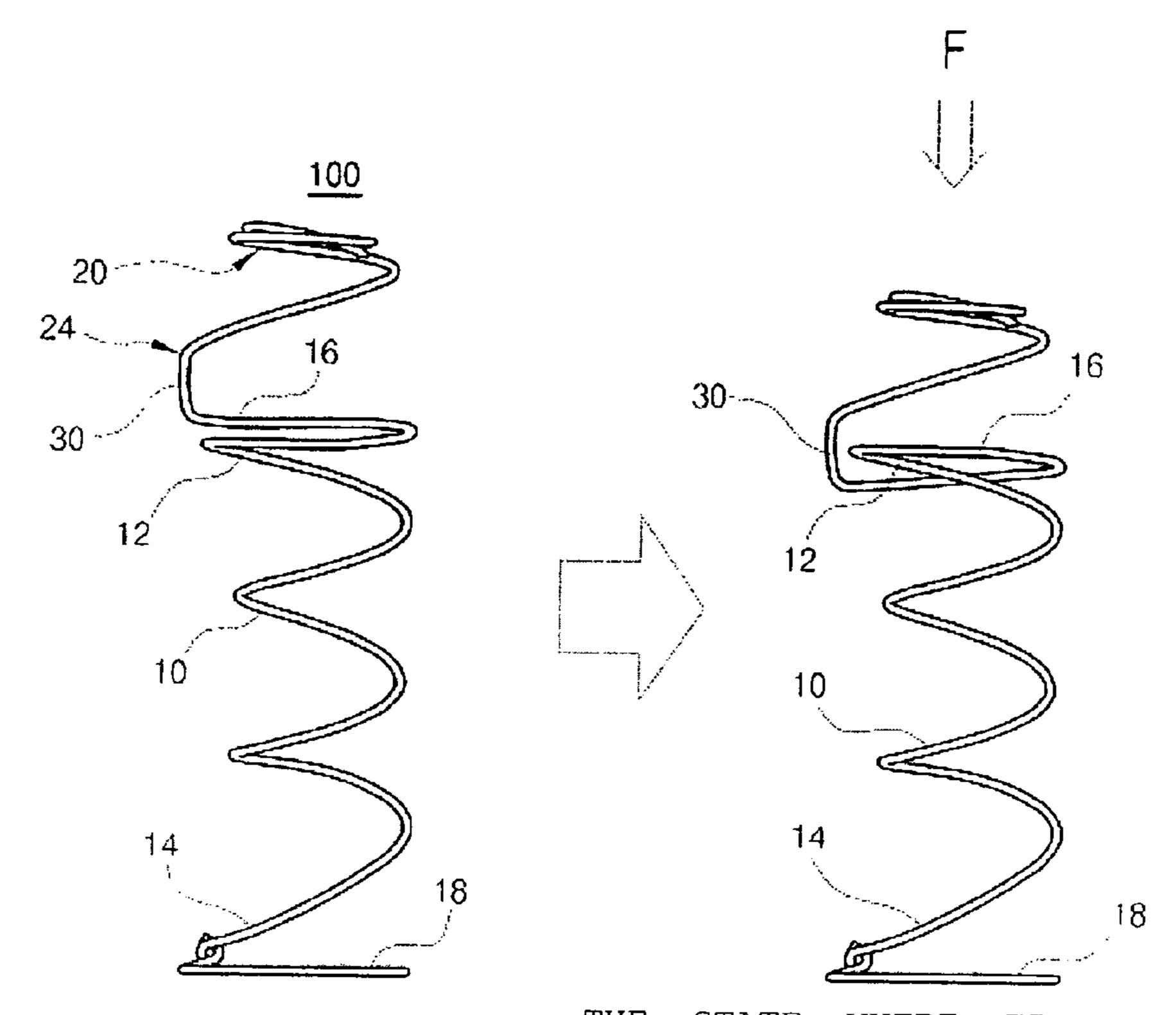
THE STATE WHERE FIRST CONTACT-PREVENTING/RIGIDITY-REINFORCING END 30 DESCENDS WITHOUT TOUCHING THE UPPERMOST WINDING 12
