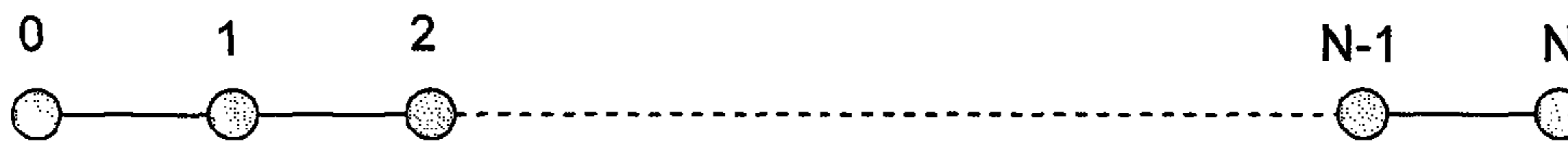
Figure 20. Linear topology with nodes being reprogrammed using Freshet and Deluge starting with node 0 as the originator ( N=1,2,\dots,16 )
