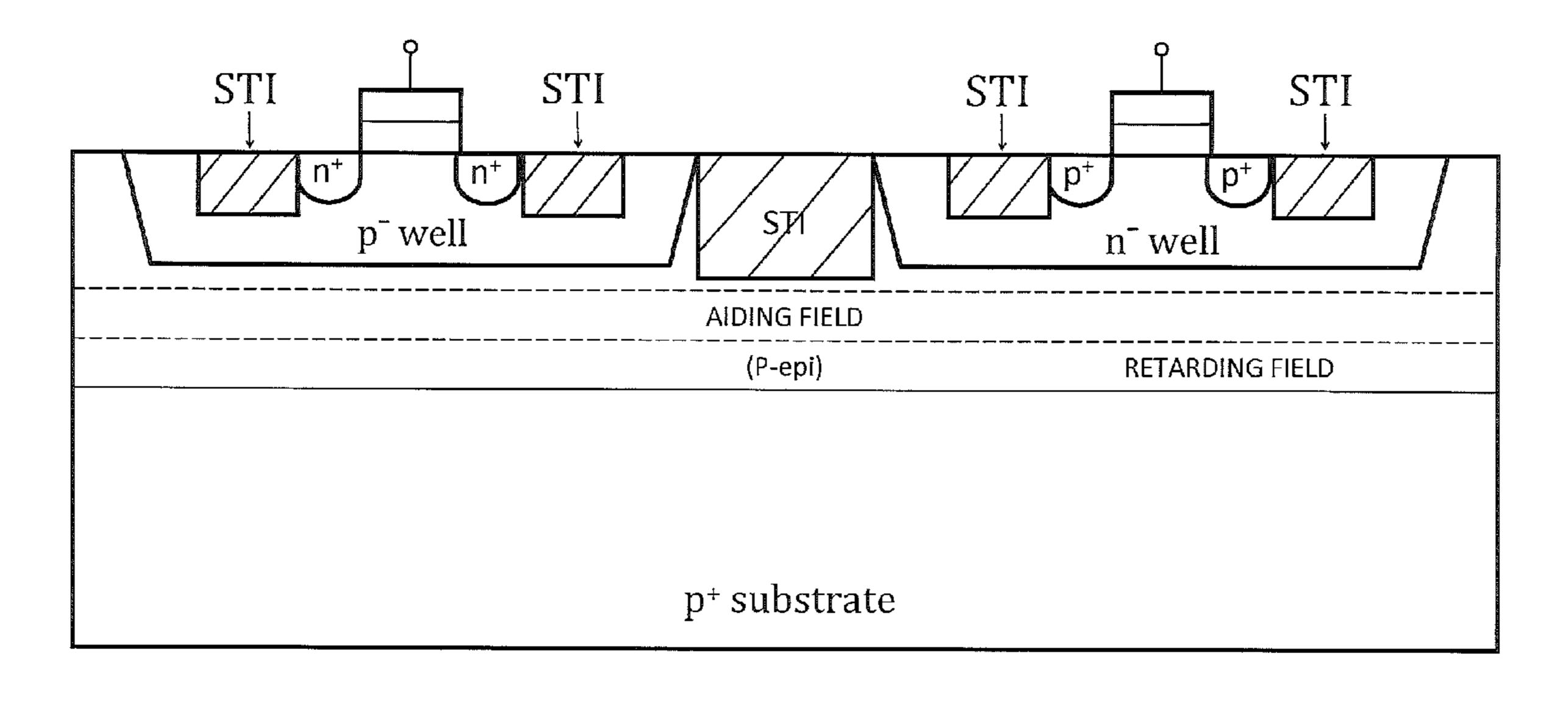
(CMOS integrated circuit built on 2-way graded dopant epitaxial layer.)
