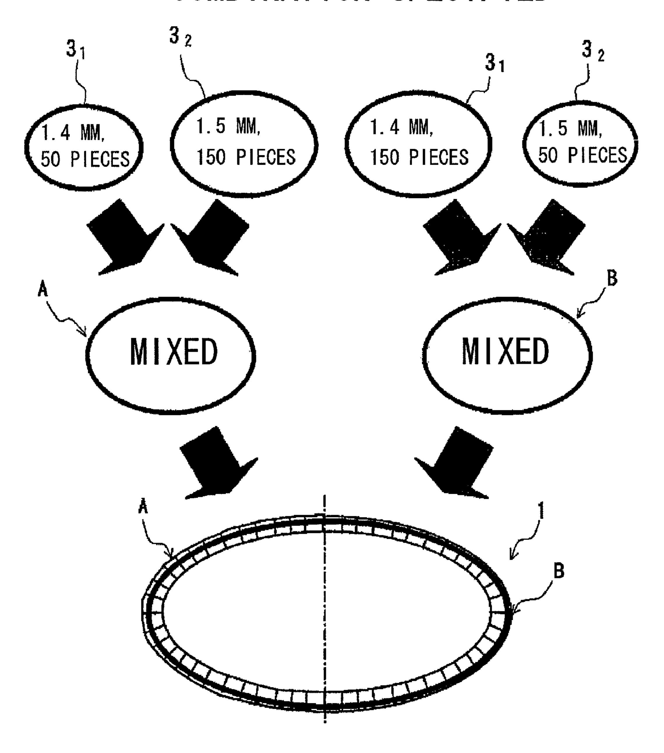
RATIO OF ELEMENTS OF 1.4 MM AND 1.5 MM IS INTENTIONALLY ADJUSTED ON RIGHT AND LEFT SIDES OF BELT
