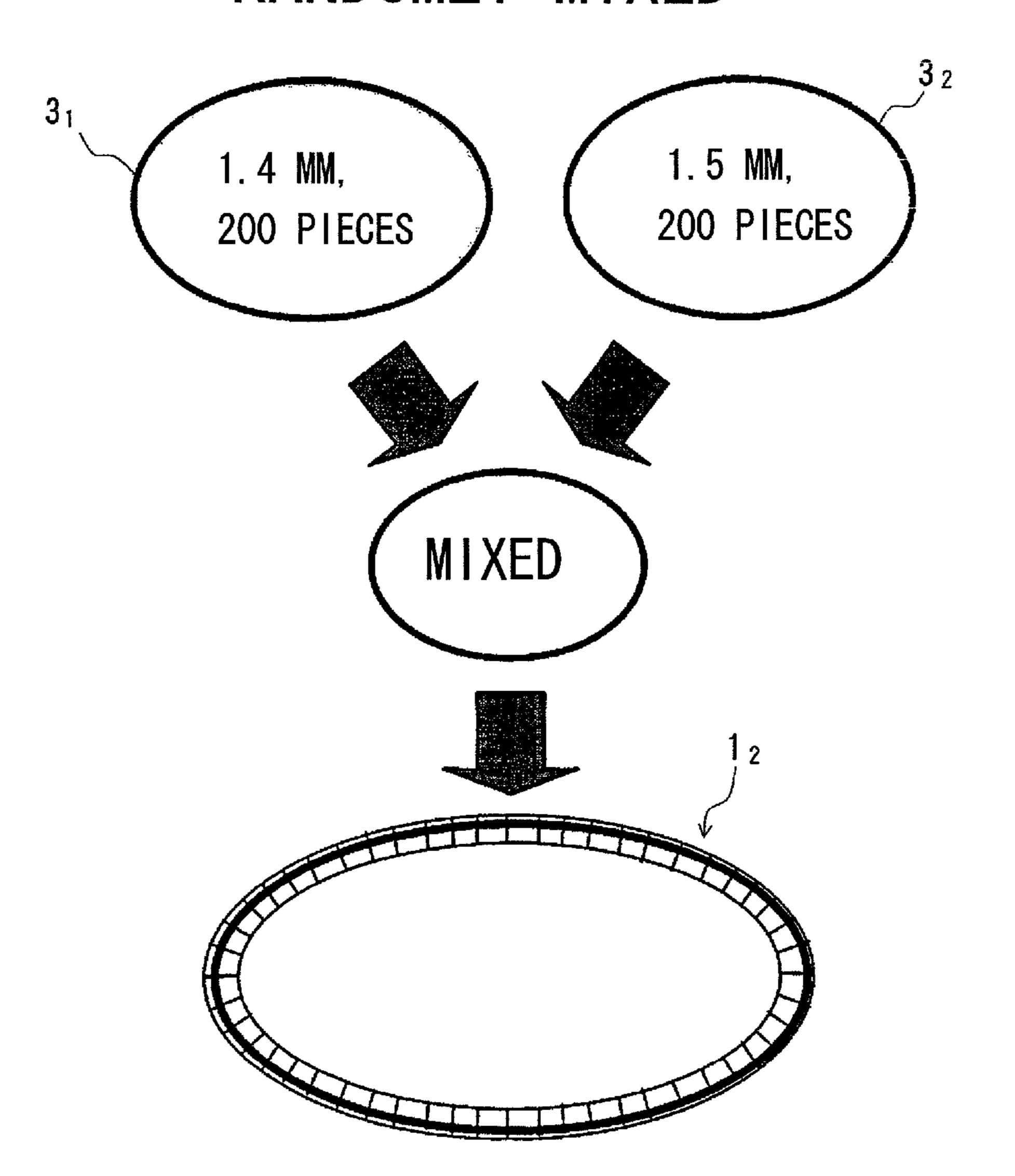
ELEMENTS OF 1.4 MM AND 1.5 MM ARE DISPOSED AT RANDOM IN WHOLE RANGE OF BELT
