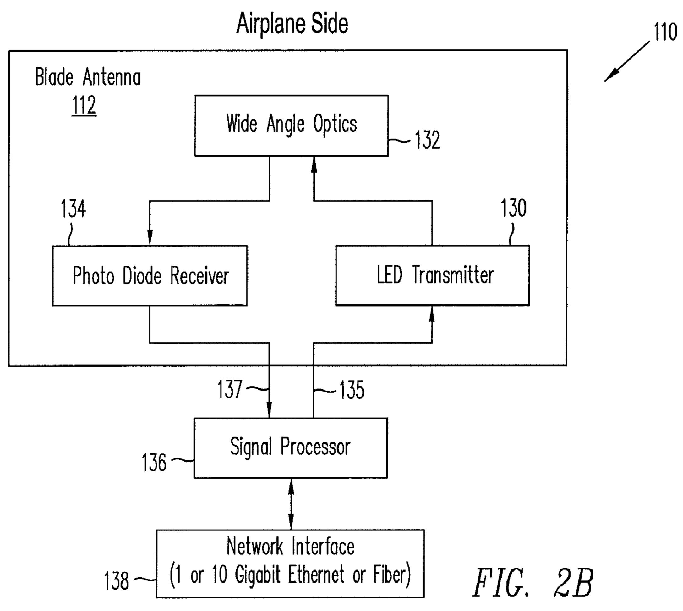
Transmitting ground—to—aircraft data at a higher bandwidth using laser light and a narrow beam width from a ground side device to an aircraft side device
