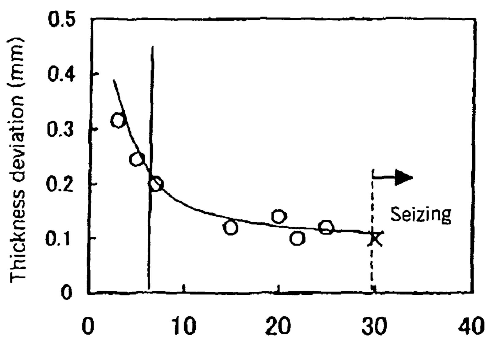
Reduction ratio of wall thickness by drawing (%)
