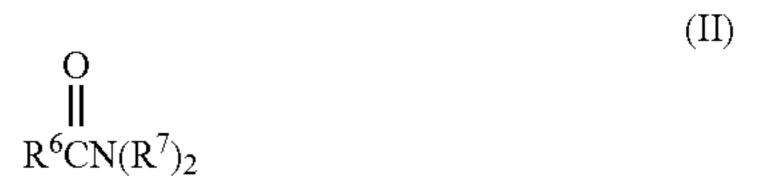
wherein  $R^6$  of formula (II) is an alkyl group containing from 7 to 21, preferably from 9 to 17, carbon atoms and each  $R^7$  of formula (II) is selected from the group consisting of hydrogen,  $C_1$ - $C_4$  alkyl,  $C_1$ - $C_4$  hydroxyalkyl, and  $-(C_2H_4O)_xH$  where x of formula (II) varies from 1 to 3. Preferred amides are  $C_8$ - $C_{20}$  ammonia amides, monoethanolamides, diethanolamides, and isopropanolamides.
