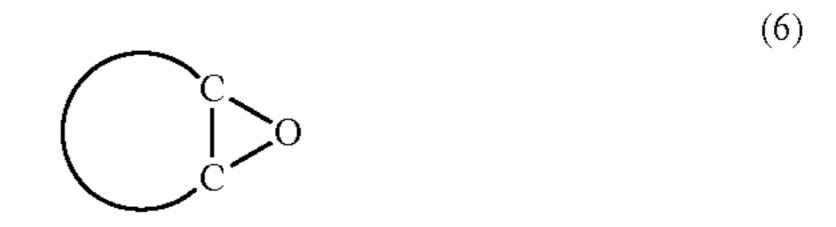
Specific examples of alicyclic epoxy compounds include 1,2-epoxycyclohexane, 1,2-epoxycyclopentane, 3,4-epoxycyclohexylmethyl-3,4-epoxycyclohexane carboxylate, bis(3, 4-epoxycyclohexylmethyl) adipate, exo-2,3-epoxynorbornane, bis(3,4-epoxy-6-methylcyclohexylmethyl)adipate, 2-(7-oxabicyclo[4.1.0]hept-3-yl)-spiro(1,3-dioxane-5,3'-[7] oxabicyclo[4.1.0]heptane, 4-(1'-methylepoxyethyl)-1,2-epoxycyclohexane, and 4-epoxyethyl-1,2-epoxycyclohexane.
