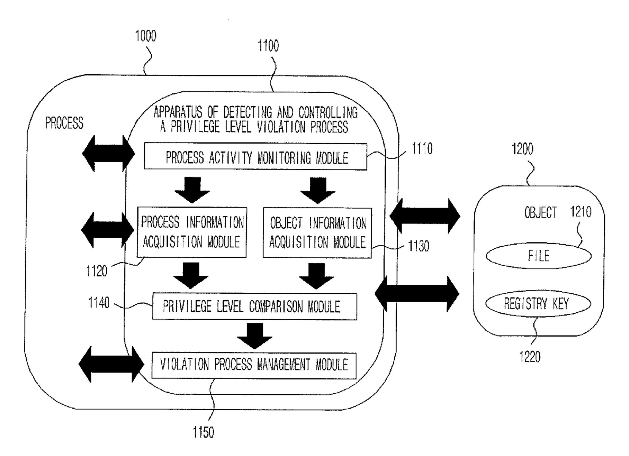
资 REGISTRY 1220 1200 OBJECT INFORMATION ACQUISITION MODULE INFORMATION APPARATUS OF DETECTING AND CONTROLLING A PRIVILEGE LEVEL VIOLATION PROCESS MODULE ACTIVITY MONITORING MODULE COMPARISON MODULE MANAGEMENT 1100 **PROCESS** INFORMATION ACQUISITION MODULE PRIVILEGE 1150 VIOLATION **PROCESS PROCESS** 1000 1140 1120 **PROCESS**
