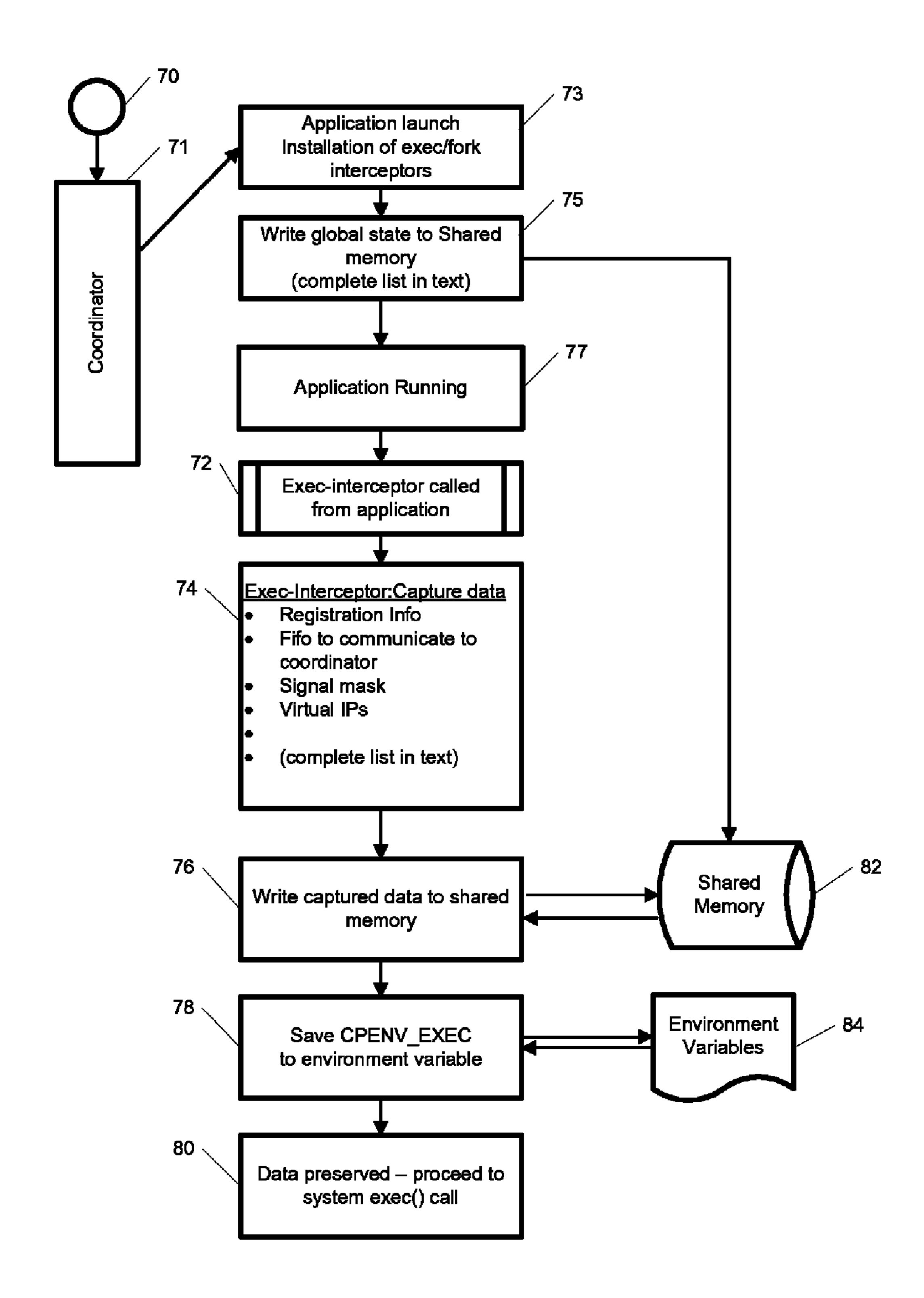
Fig. 3 – Exec-Interceptor Mechanism to capture and preserve information across exec
