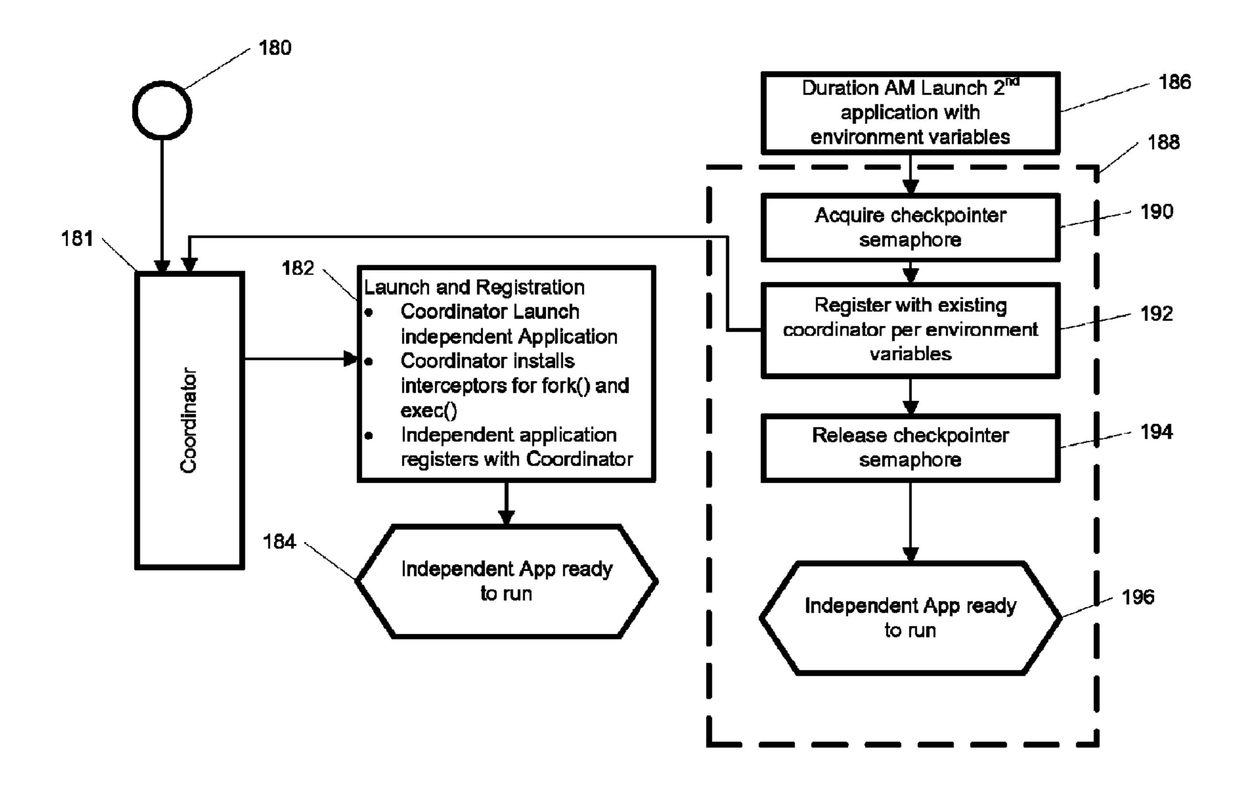
Fig.6 – Launch and Registration of independently Launched Applications
