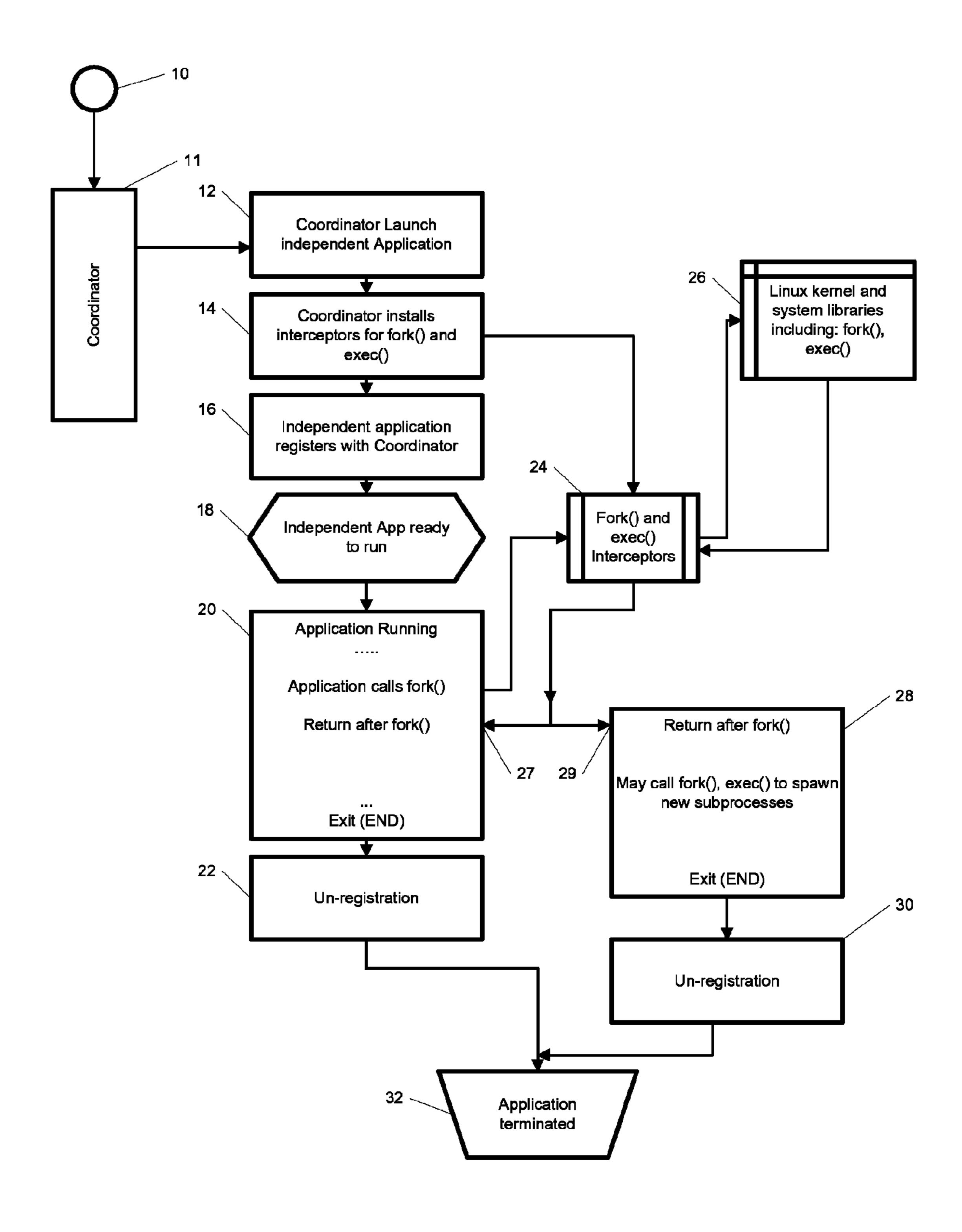
Fig. 1 – Core operation of fork()
