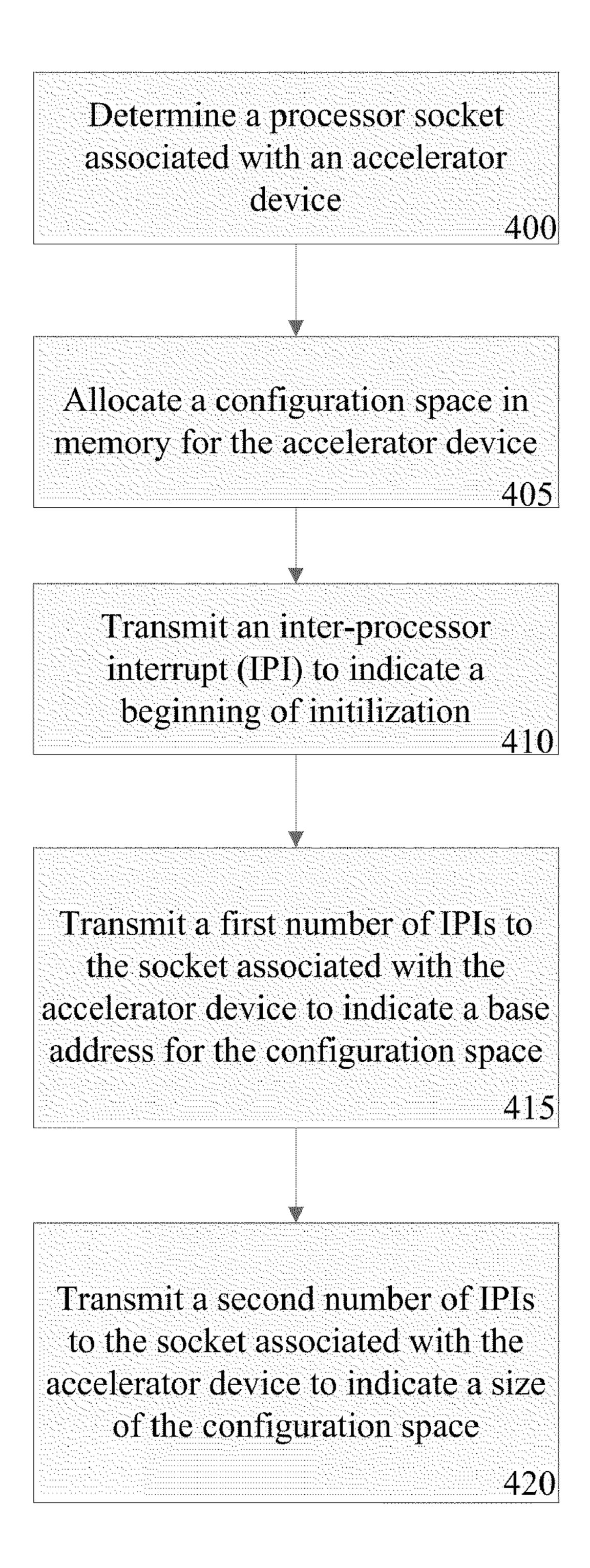
Execute reconfiguration code on a physical processor in a socket of computer system
