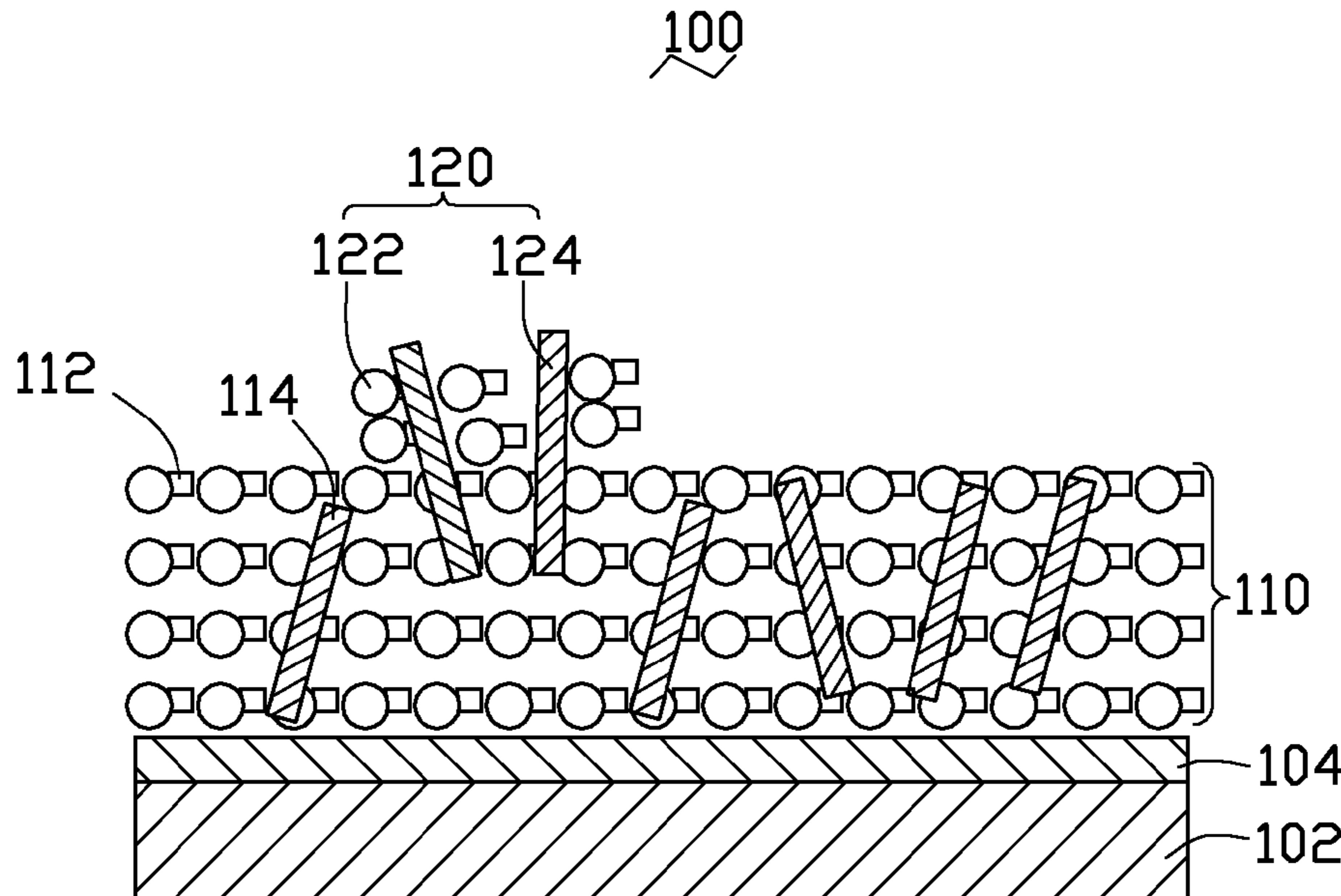
providing a substrate, and depositing a cathode layer on a surface of the substrate
