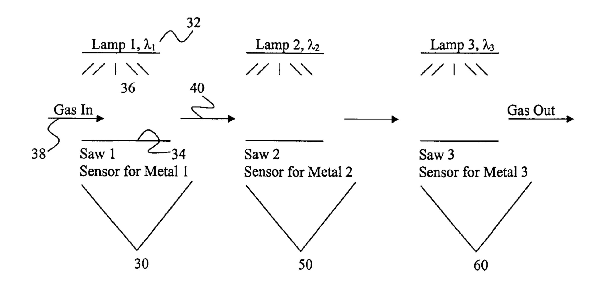
Figure 3: Array of Photodeposition Detectors for Determination of Metals in a Gas Stream
