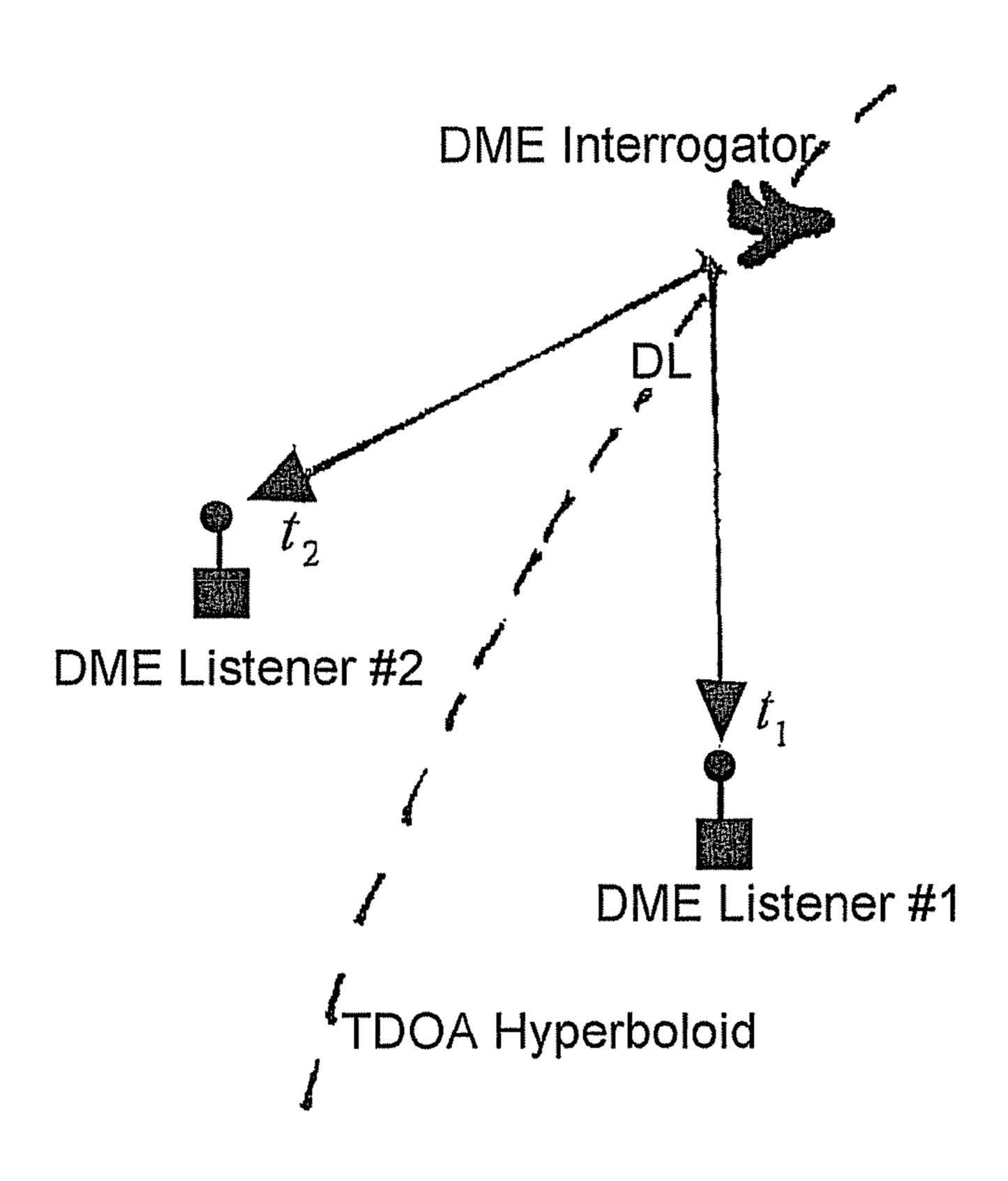
TDOA =  $t_2 - t_1$ obtained by XCORR {DL@Listener #1, DL@Listener #2}
