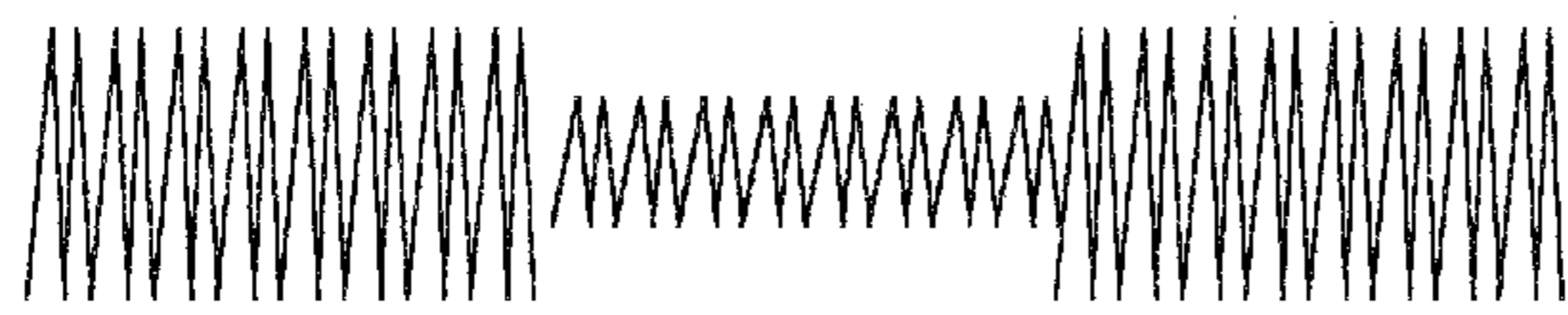
a) 4 Cycles per bit reduced amplitudes for 0 states
