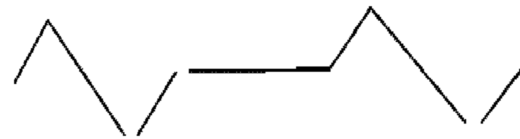
b) Single cycle per bit with zero transmit for 0 State
