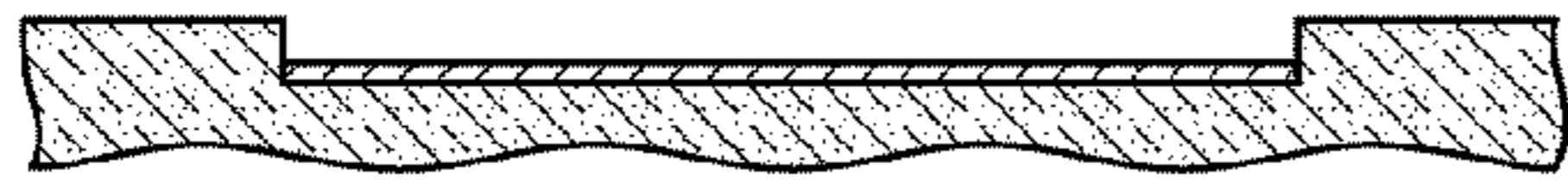
Recess & Shield Metal Layer
