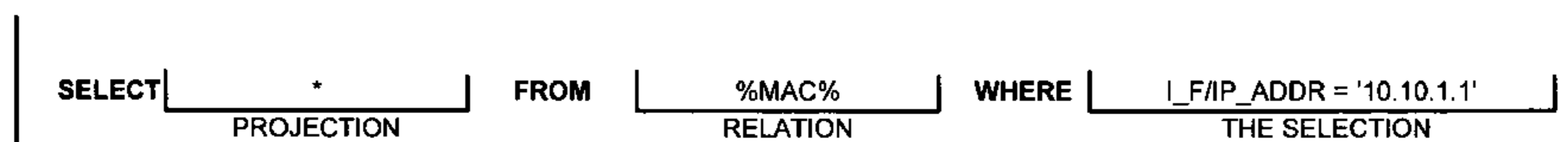
SINGLE QUERY WITH UNSTRUCTURED SEARCH STRING WITHIN A STRUCTURED SEARCH QUERY EXAMPLE THAT INCLUDES A WHERE CLAUSE
