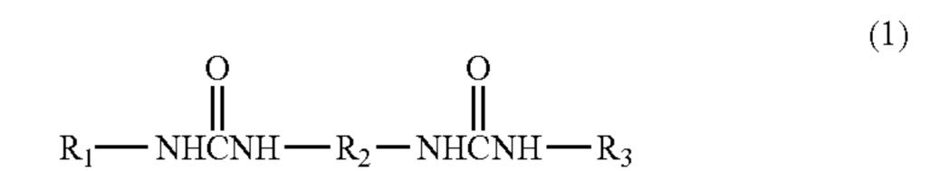
where  $R_1$  and  $R_3$  are a straight-chain alkyl groups having 9 to 22 carbon atoms respectively, and  $R_2$  is an aromatic hydrocarbon group having 6 to 15 carbon atoms. The lubricant composition is sealed into the rolling bearing.
