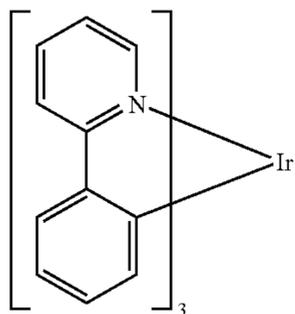
In this, and later figures herein, we depict the dative bond from nitrogen to metal (here, Ir) as a straight line. Ir(ppy)<sub>3</sub> emits a spectrum at CIE 0.30, 0.63, and has a half-life of about 10,000 hours at an initial luminance of 500 cd/m<sup>2</sup>, and a quantum efficiency of about 6%. Kwong et al., *Appl. Phys. Lett.*, 81, 162 (2002).
