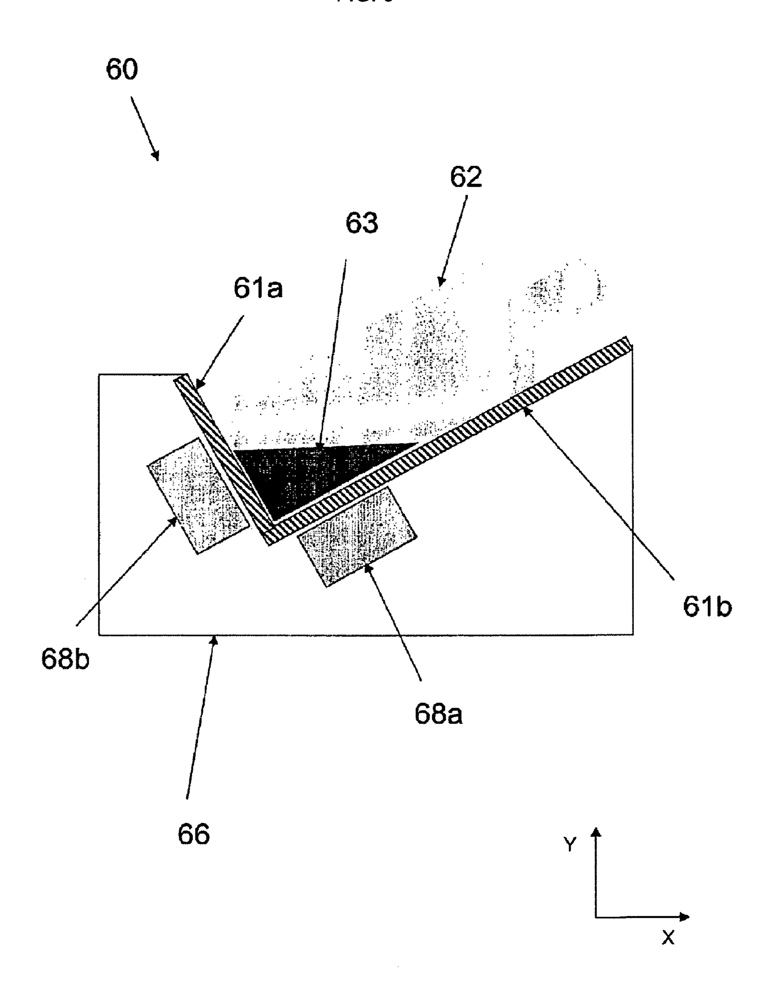
METHOD FOR IDENTIFYING A SAMPLE IN A CONTAINER, E.G. WHEN CONDUCTING A TRAVELER SURVEY IN THE CHECK-IN AREA, BY DETERMINING THE RESONANCE FREQUENCY AND THE QUALITY OF A DIELECTRIC RESONATOR TO WHICH THE CONTAINER IS ARRANGED
