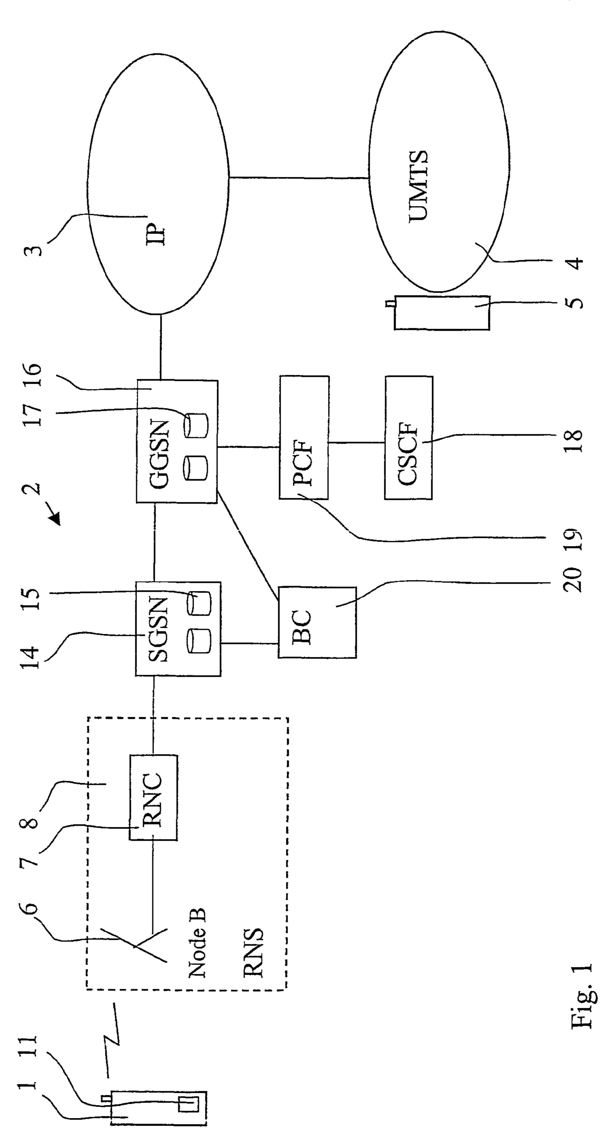
Initiate call set-up procedure for a voice over IP connection for a user equipment via a communication system
