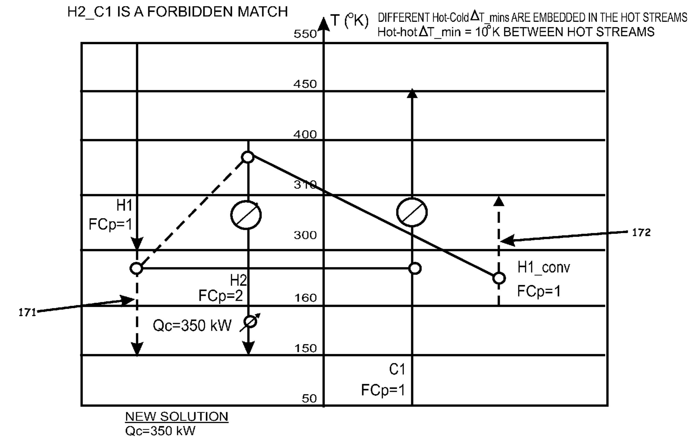
FIG. 34. Qh=0.0 kW SAME NUMBER OF HEAT EXCHANGERS
