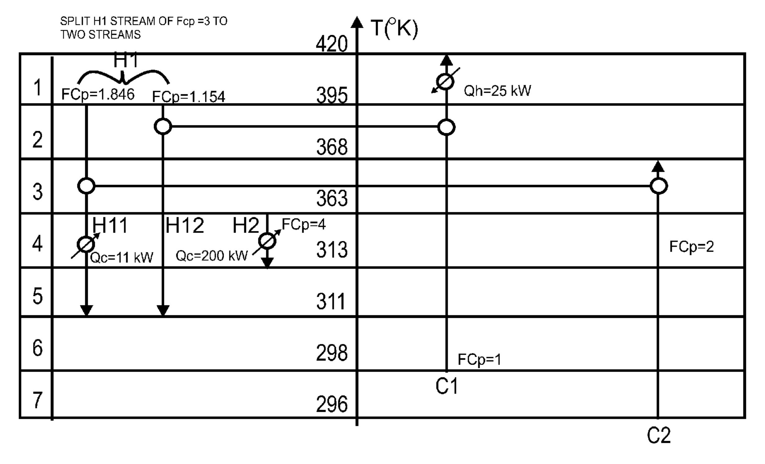
FIG. 27. NUMBER OF HEAT EXCHANGERS USED IS 5.
