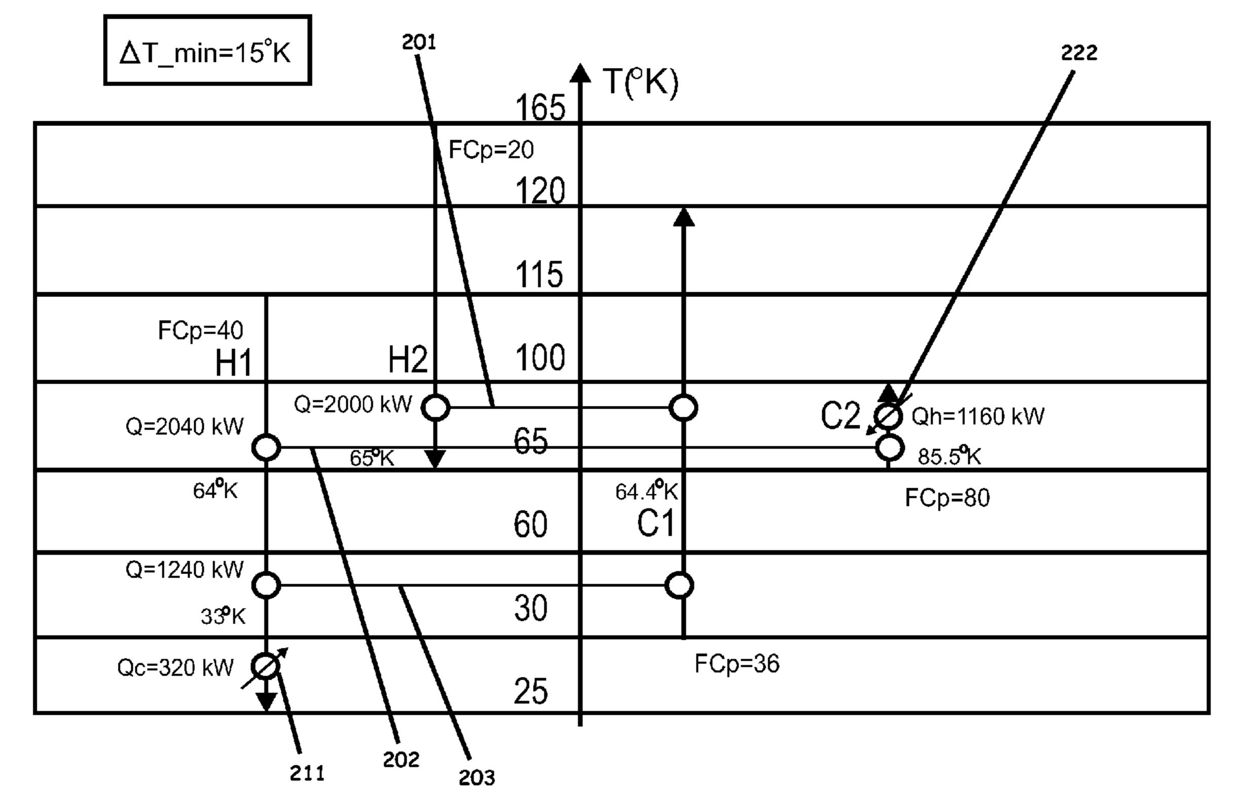
FIG. 41. -THREE PROCESS-TO-PROCESS HEAT EXCHANGERS, BUT ONLY ONE COOLER AND ONE HEATER -SAME STRUCTURE BUT DIFFERENT LOADS.
