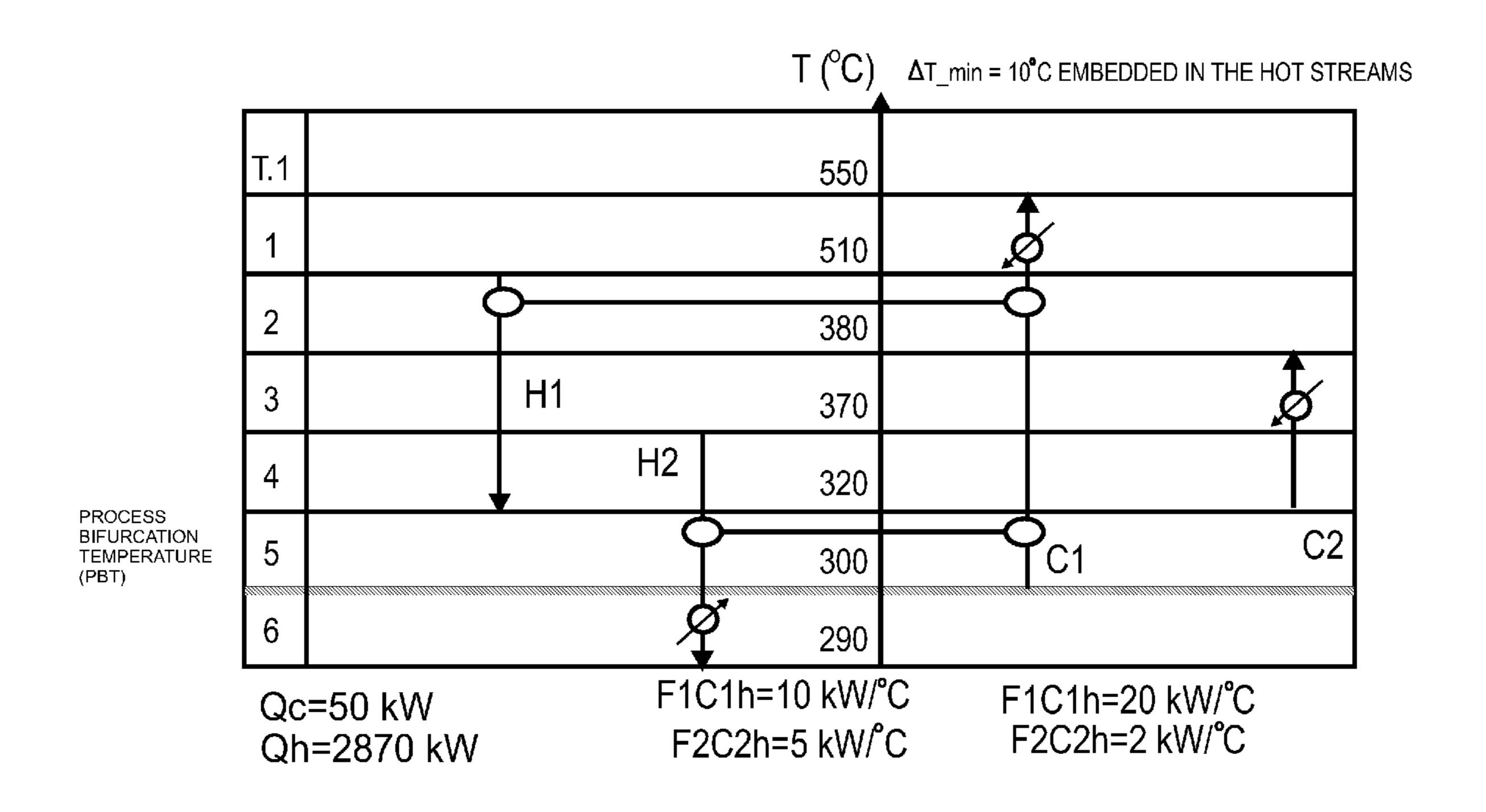
FIG. 14. NUMBER OF HEAT EXCHANGERS USED IS 5.
