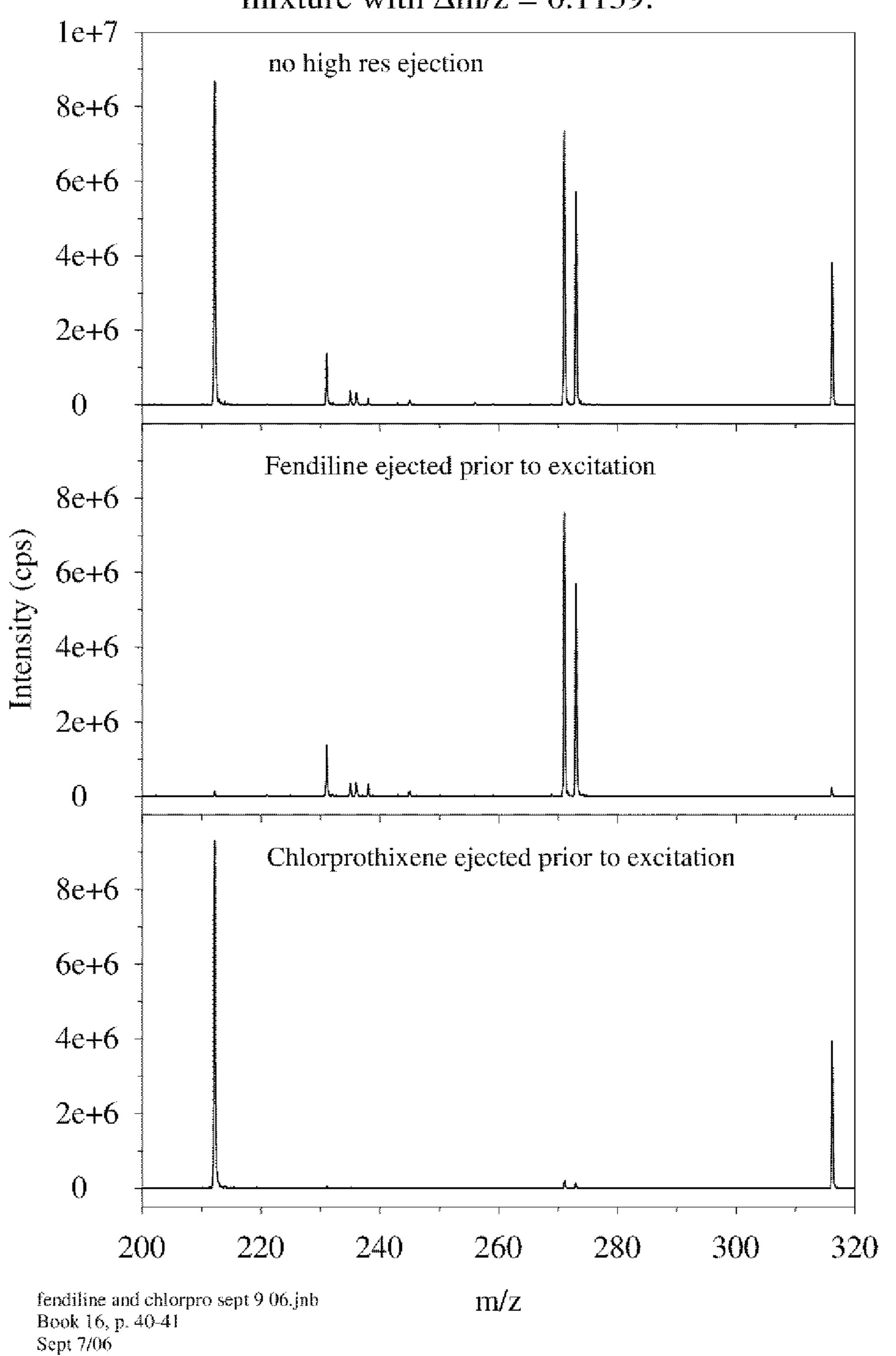
FIG. 5 Oxycodone (316.1543 m/z) and Chlorprothixene (316.0921 m/z) mixture with  $\Delta m/z = 0.0622$ .
