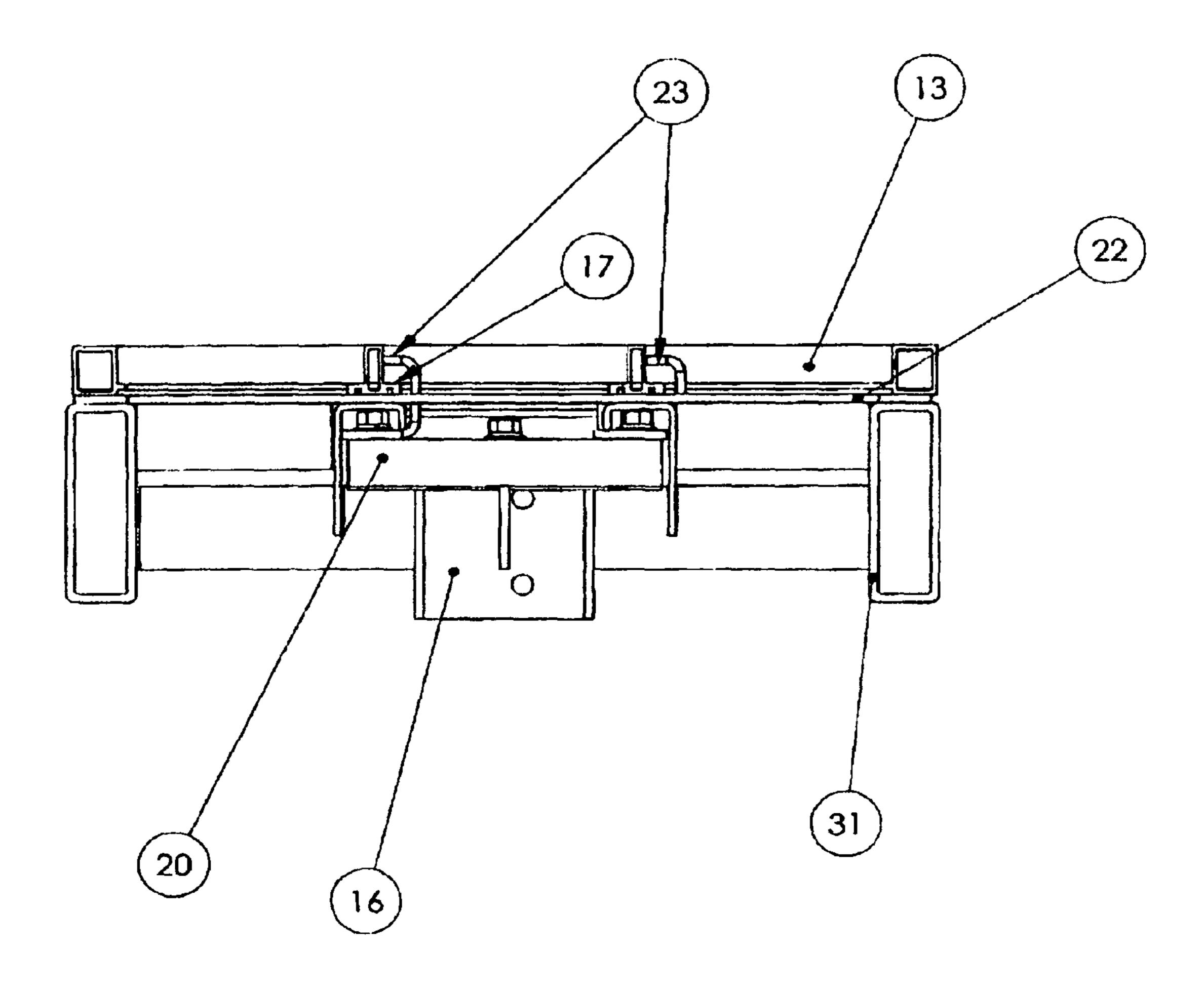
Figure 8: Screen Remove - step 1: Screen Clamp up
