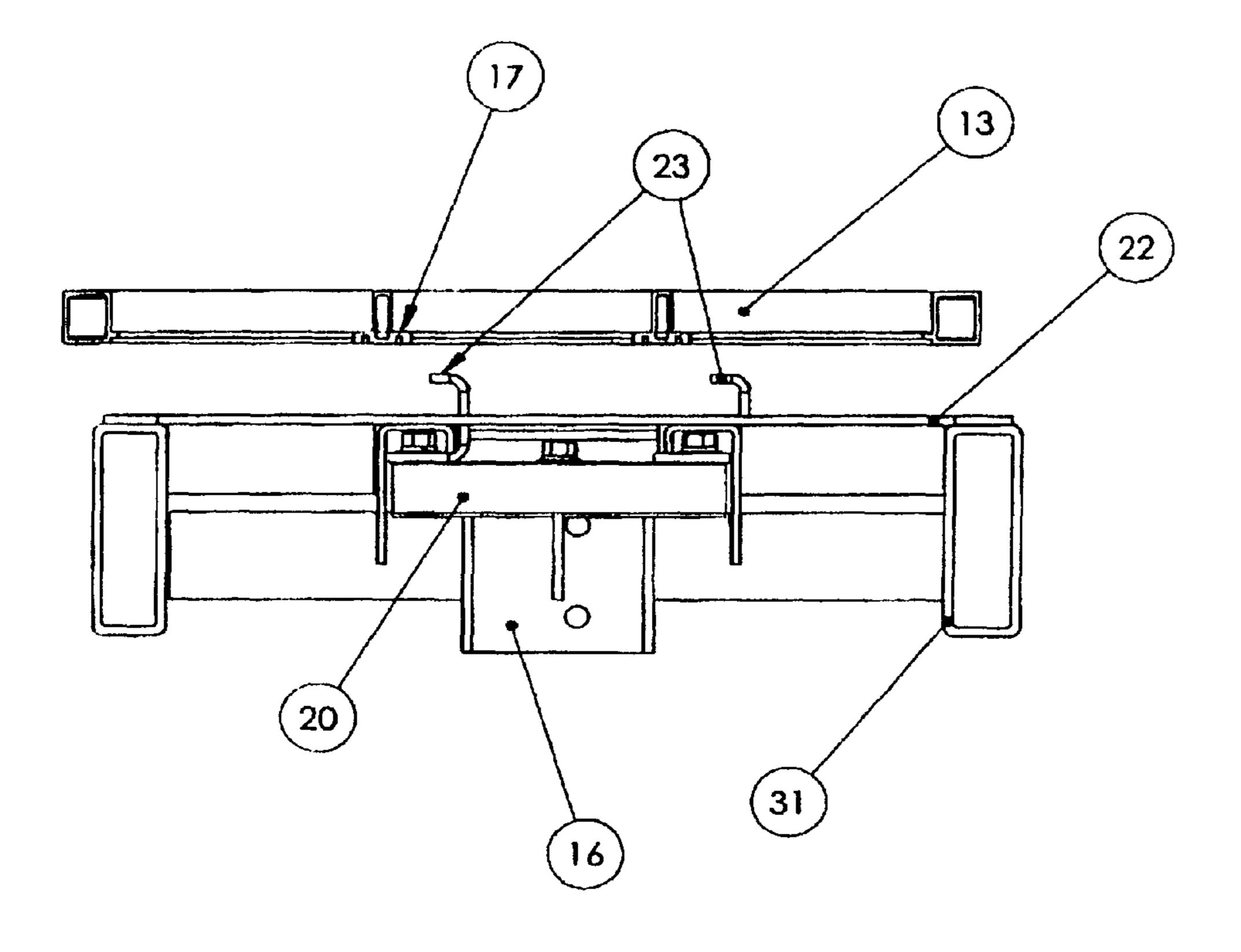
Figure 10: Screen Remove- step 3: Screen Clamp up, Screen Frame moved left away from Clamp Finger Plate and up for removal
