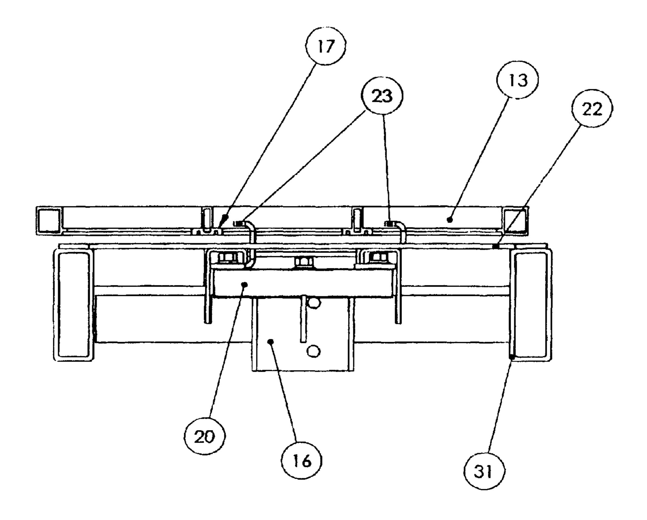
Figure 9: Screen Remove - step 2: Screen Clamp up, Screen Frame moved left away from Clamp Finger Plate
