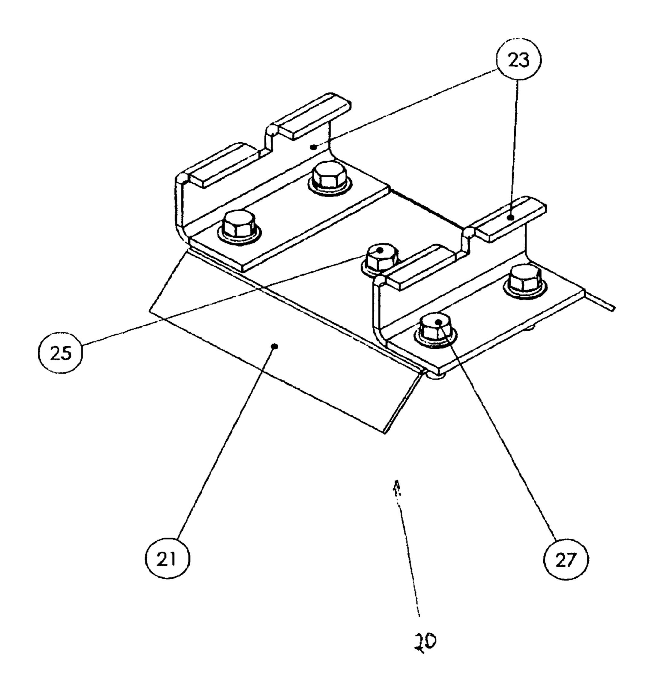
Figure 6: Screen Clamp Assembly
