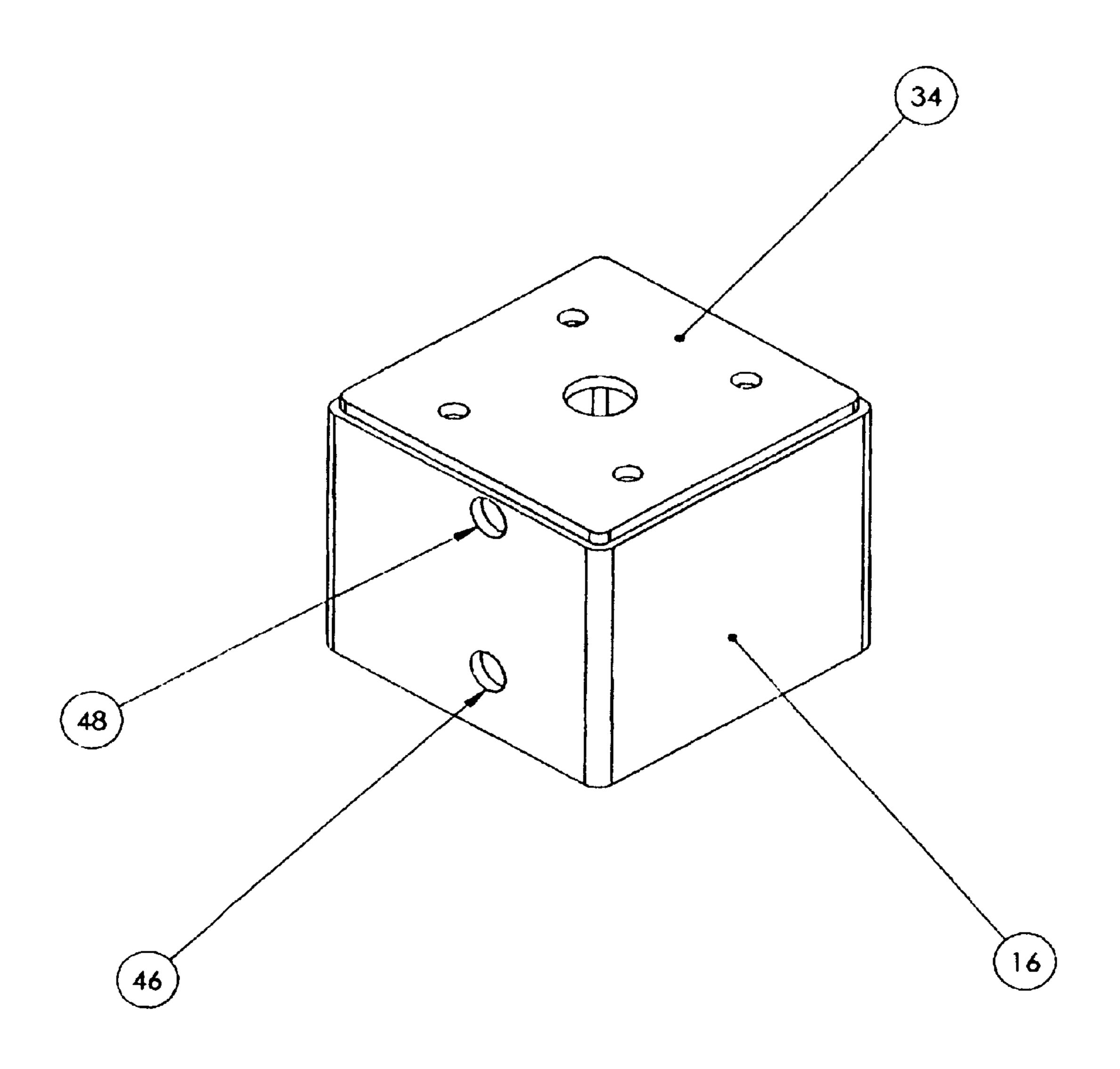
Figure 4A: Pneumatic Cylinder Holder
