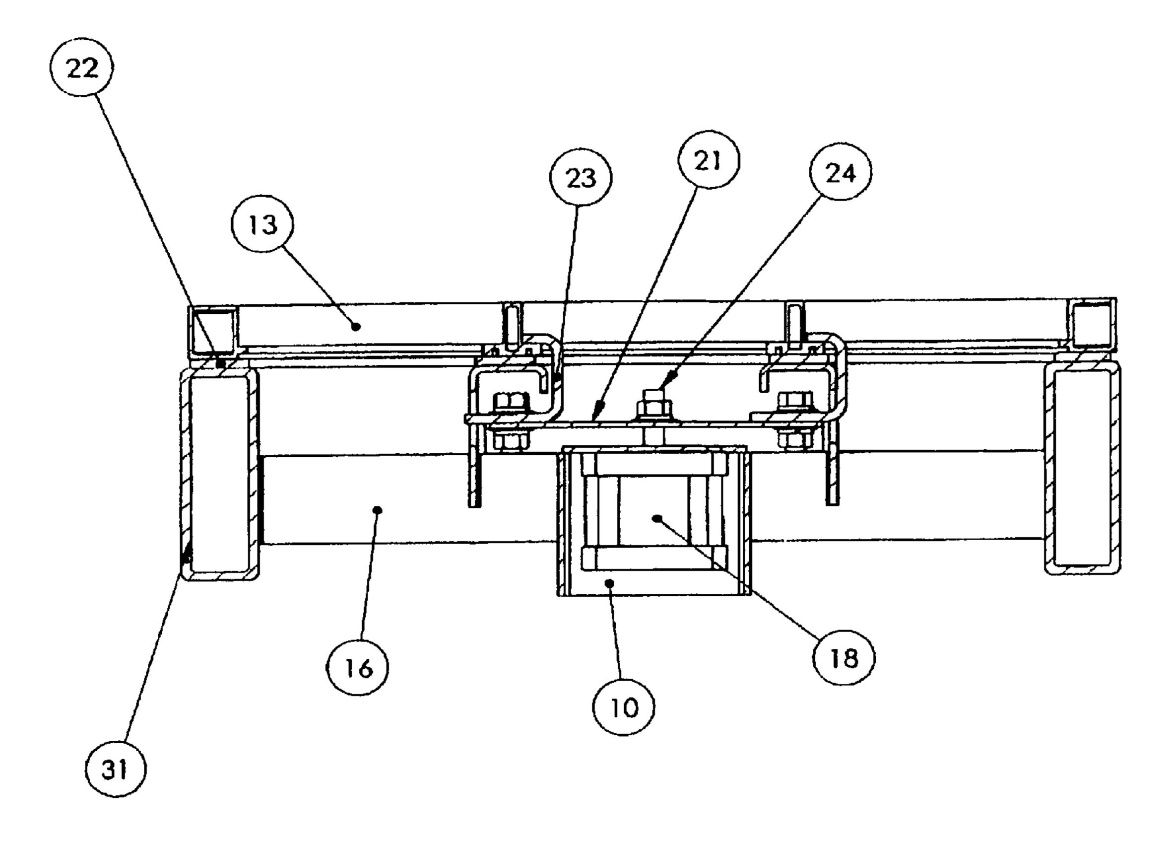
Figure 1A: Screen Bed Assembly Section
