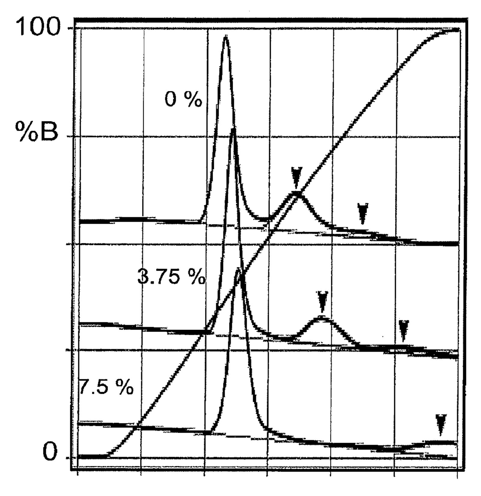
CHT I, 20  $\mu$ m 5 x 50 mm 20 CV LG, A to B 1 mL/min, 300 cm/hr chimeric IgG<sub>1</sub> (a)
