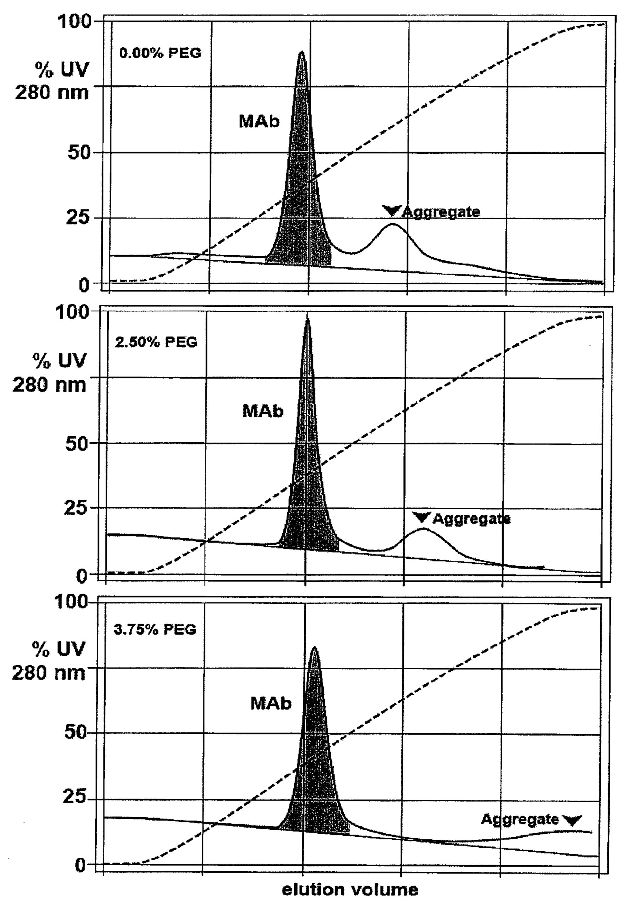
CHT Type II, 20 µm, 5 mm x 50 mm, protein A purified human IgG1 50 mL linear gradient elution from 5mM NaPO4, pH 6.7 to 5mM NaPO4, 2M NaCl, plus PEG-6000 as indicated, pH 6.7 600 cm/hr (2 mL/min)
