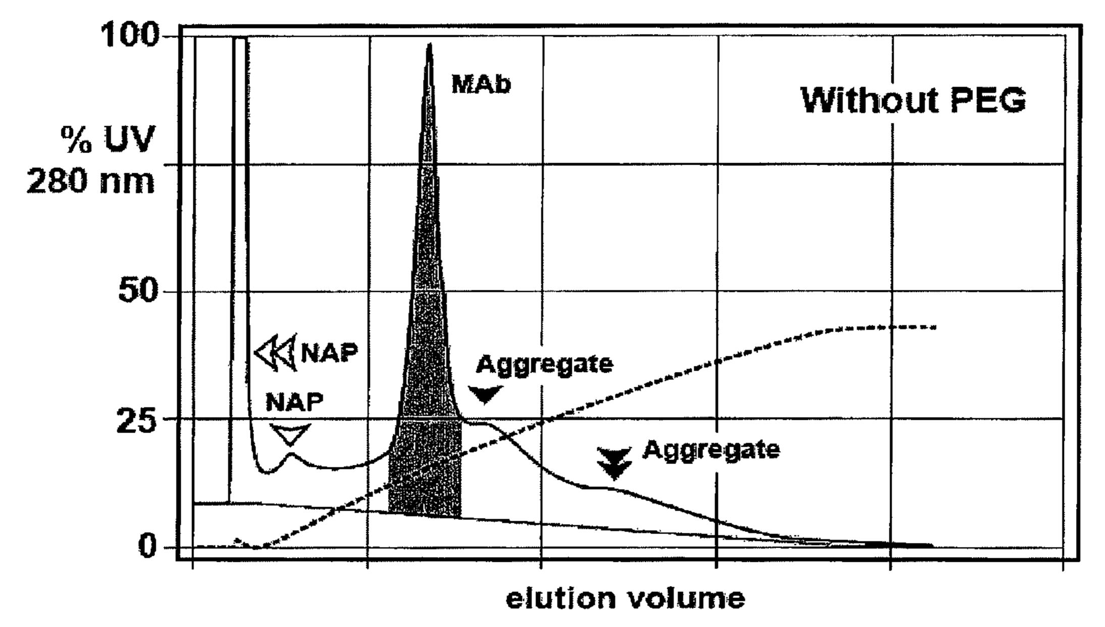
CHT Type II, 20 µm, 5 mm x 50 mm, unpurified chimeric IgG1 50 mL linear gradient elution from 5mM NaPO4, pH 6.7 to 330 mM NaPO4, pH 6.7, 300 cm/hr (1 mL/min)
