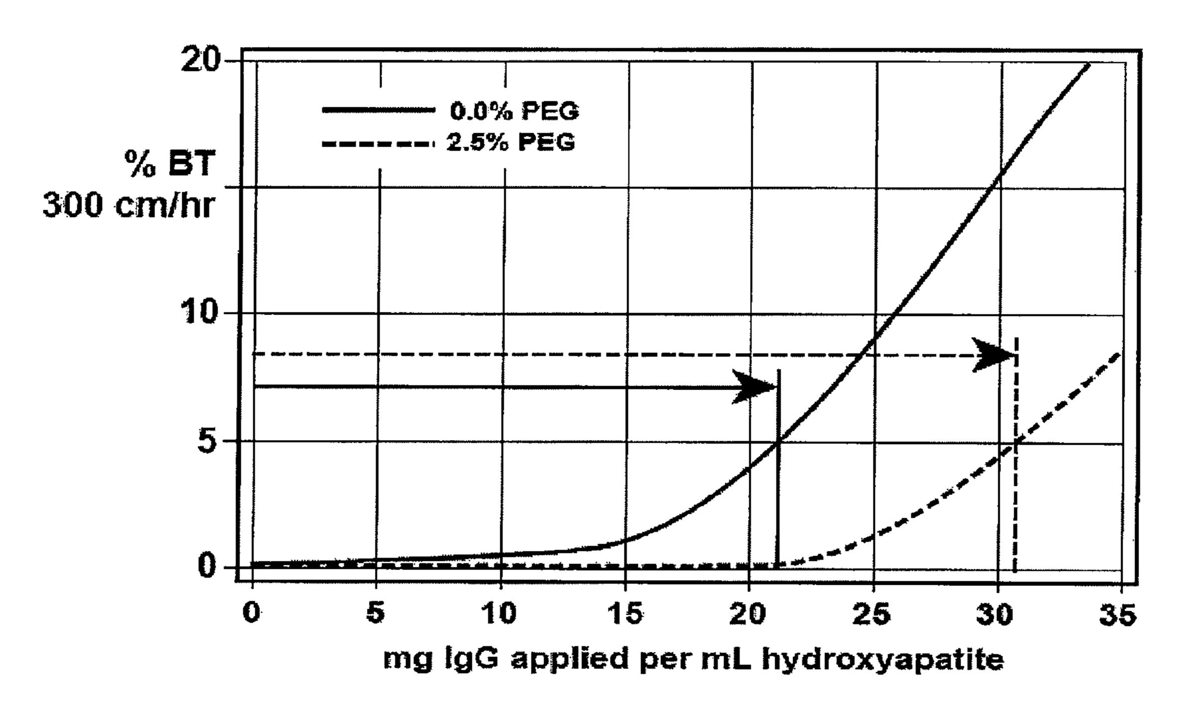
CHT Type II, 20 µm, 5 mm x 50 mm
