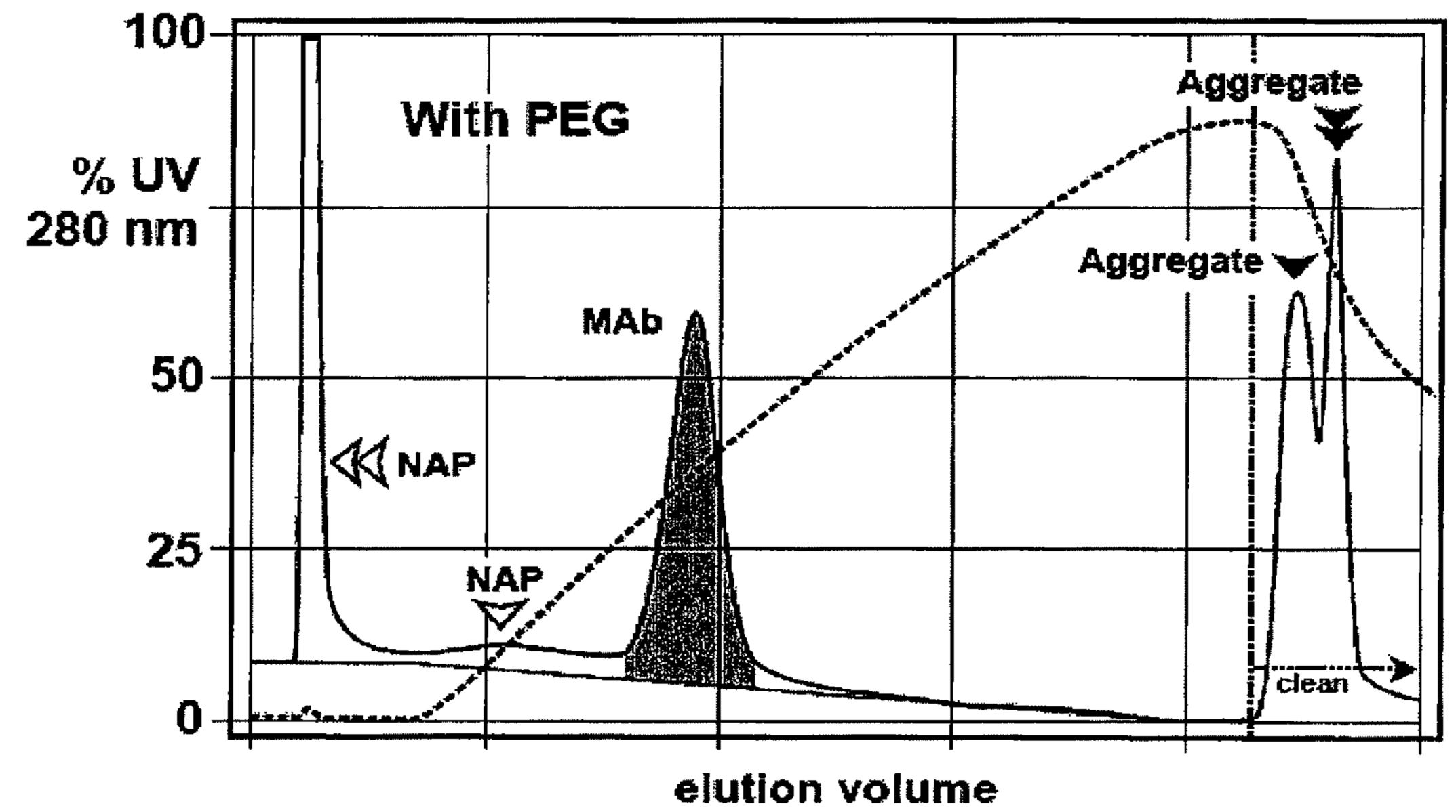
CHT Type II, 20 µm, 5 mm x 50 mm, unpurified chimeric IgG1 50 mL linear gradient elution from 5mM NaPO4, pH 6.7 to 5mM NaPO4, 2M NaCl, 5% PEG-6000, pH 6.7. Clean with 500mM NaPO4, 300 cm/hr (1 mL/min)
