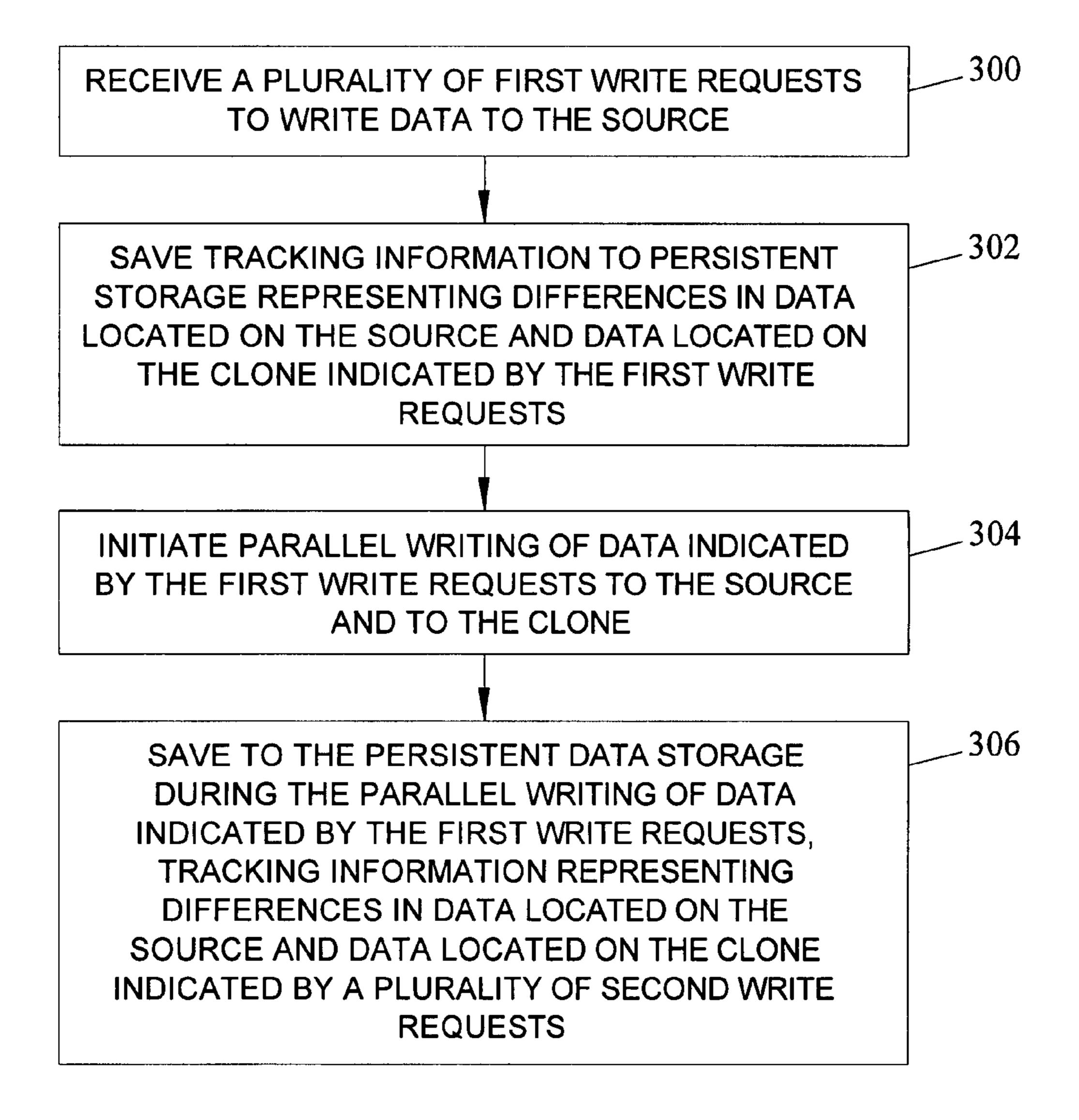
METHODS, SYSTEMS, AND COMPUTER PROGRAM PRODUCTS FOR PARALLEL PROCESSING AND SAVING TRACKING INFORMATION FOR MULTIPLE WRITE REQUESTS IN A DATA REPLICATION ENVIRONMENT INCLUDING MULTIPLE STORAGE DEVICES
