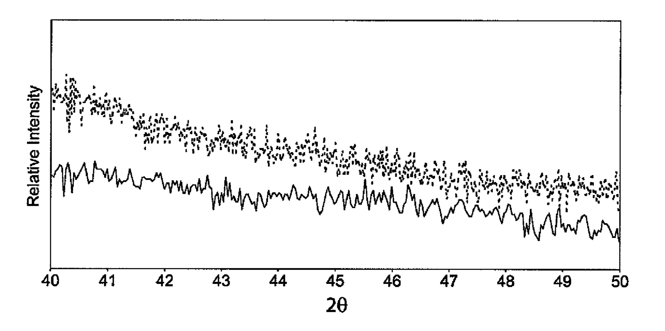
Powder x-ray diffraction pattern, not reduced (- - -) and reduced (--), of the 1.07 wt% Au(0) and Pd(0) colloidal aluminosilicate particles with a mole ratio of Pd(0)/Au(0)=4.
