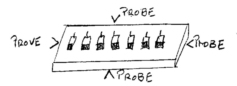
PROBES AND NETWORK ANALYZER measure resonant frequency and balance (impedance)
