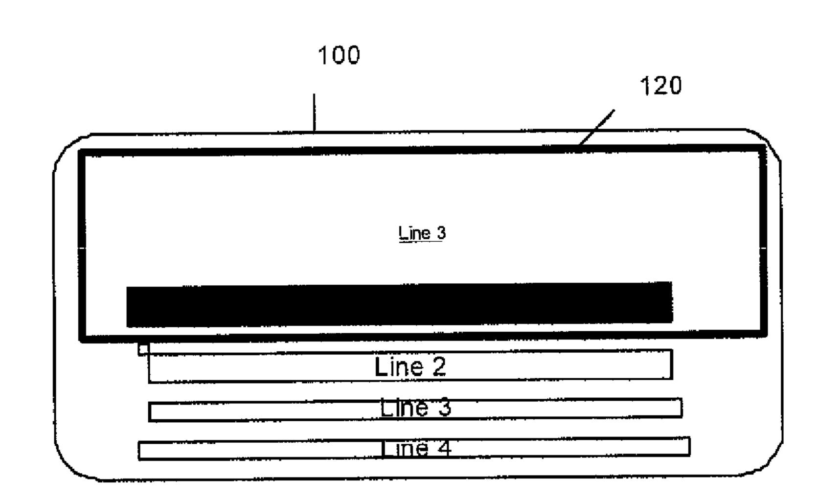
Fourth line embossing does not damage antenna 120
