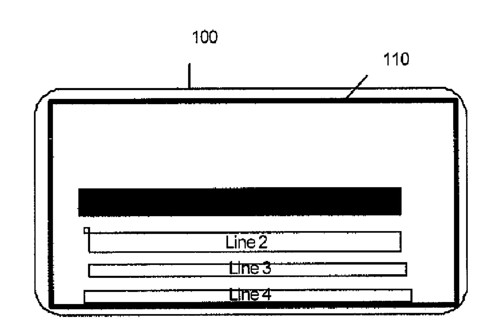
Fourth line embossing typically damages antenna 110
