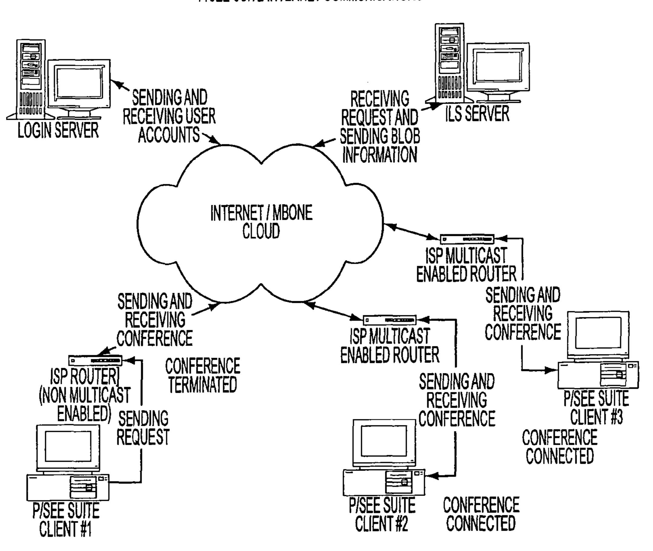
CLIENTS #2 AND #3 CAN JOIN/CREATE A CONFERENCE WITHOUT DIFFICULTY BECAUSE THEIR ISP USES A MULTICAST ENABLED ROUTER.
