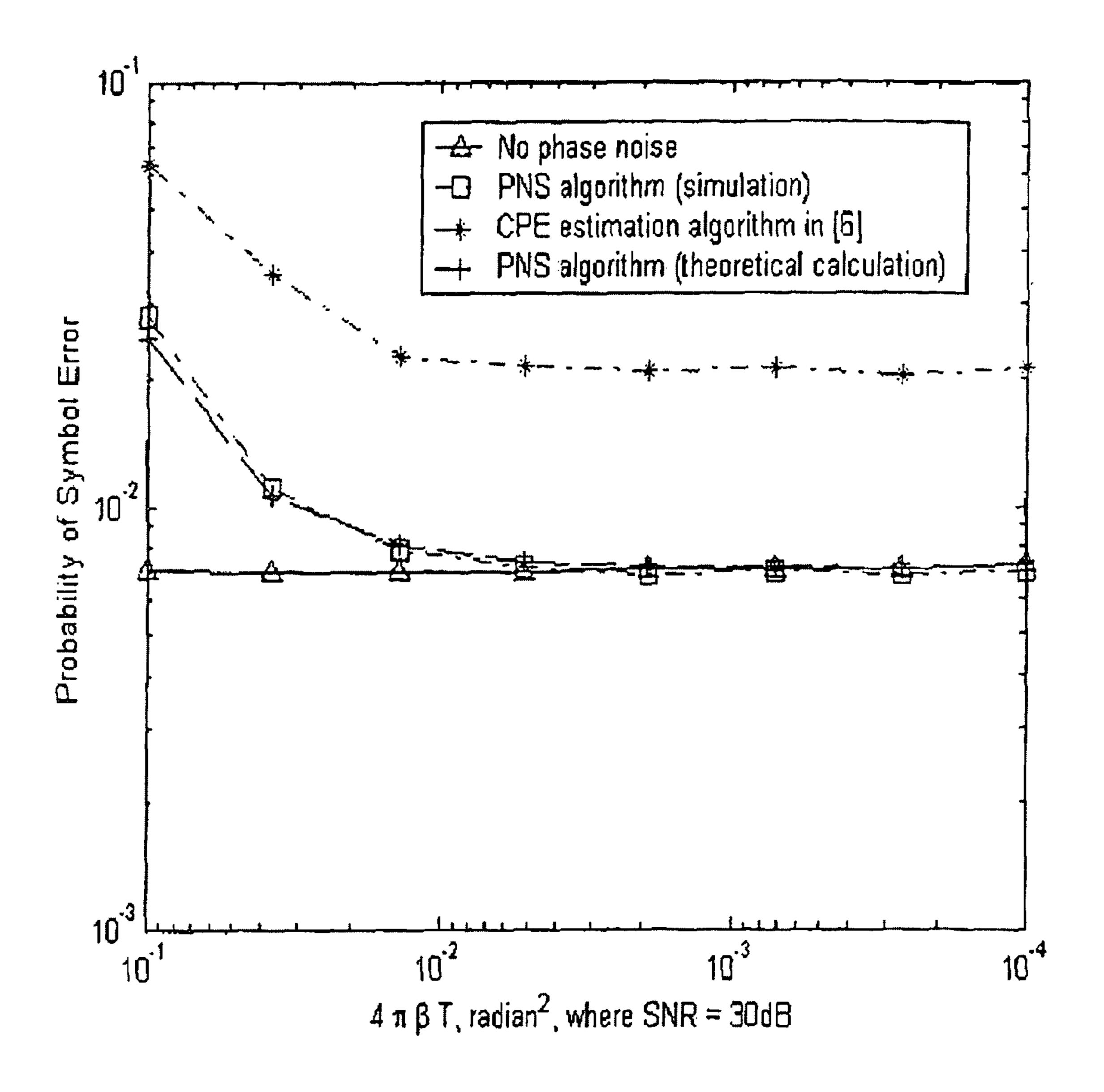
FIG. 3: PNS algorithm, symbol error probability vs. phase noise energy  $4\pi\beta T$
