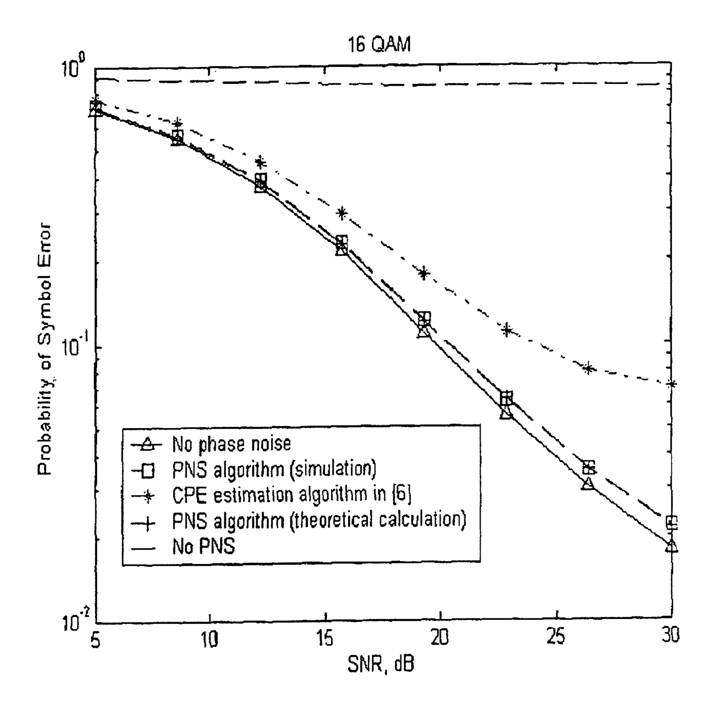
FIG. 2: PNS algorithm performance for 16QAM, with phase noise vs.  $4\pi\beta T$  equal to 0.0384 rad<sup>2</sup>
