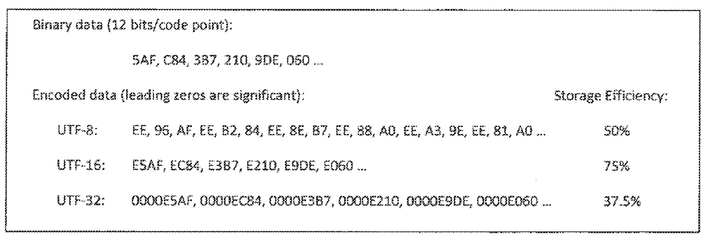
Figure 1: Present encoding method for any binary data
