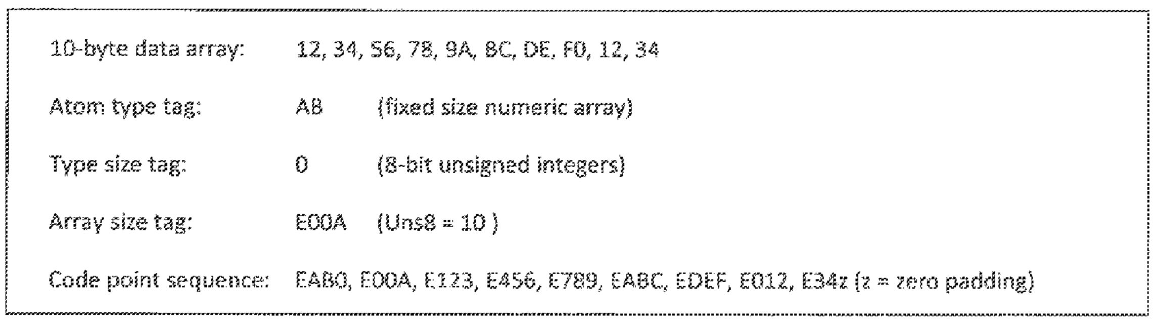
Figure 3: Present encoding method for an Unsigned Byte Array
