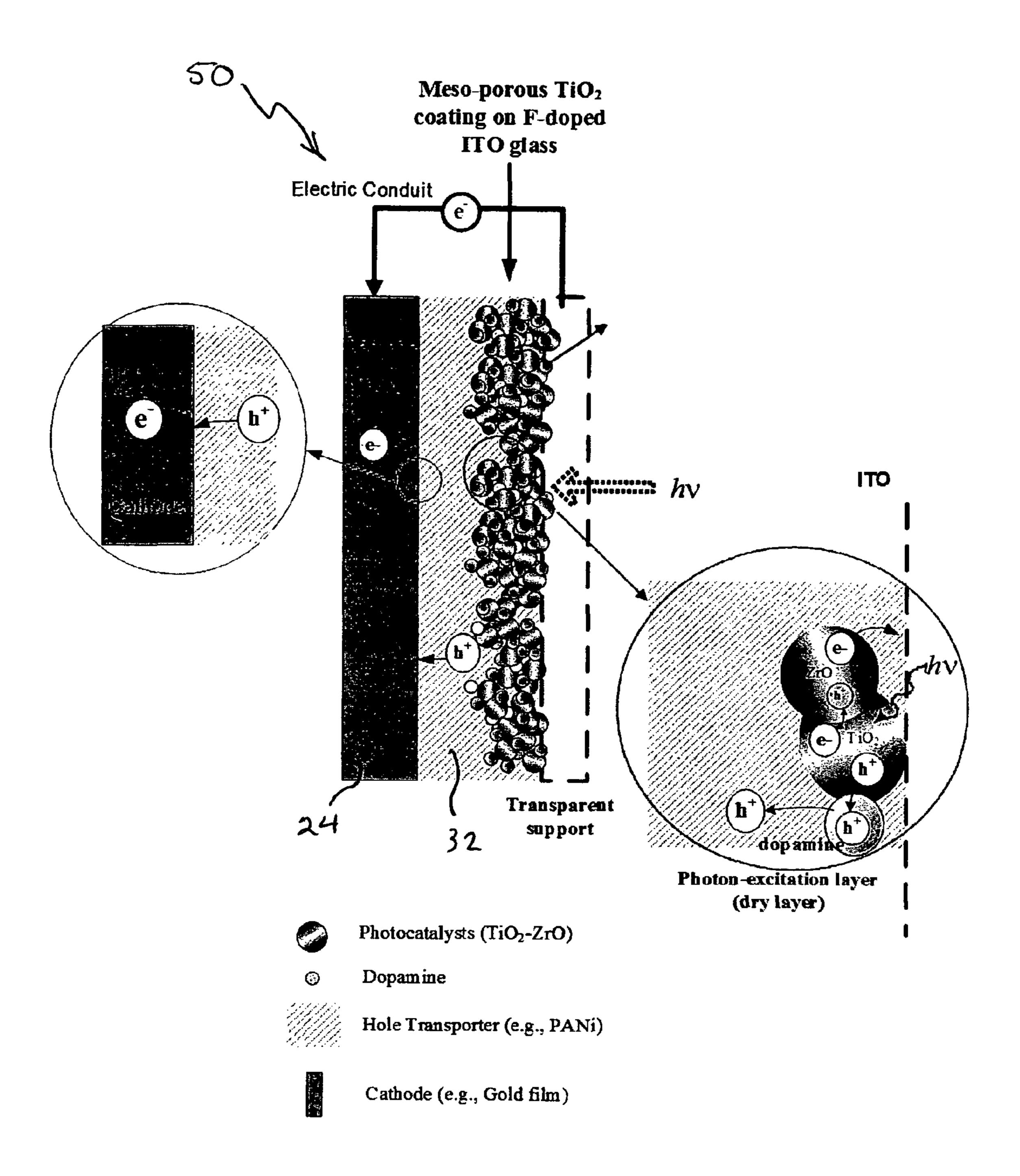
Figure 4. Configuration of Photovoltaic device to generate electricity
