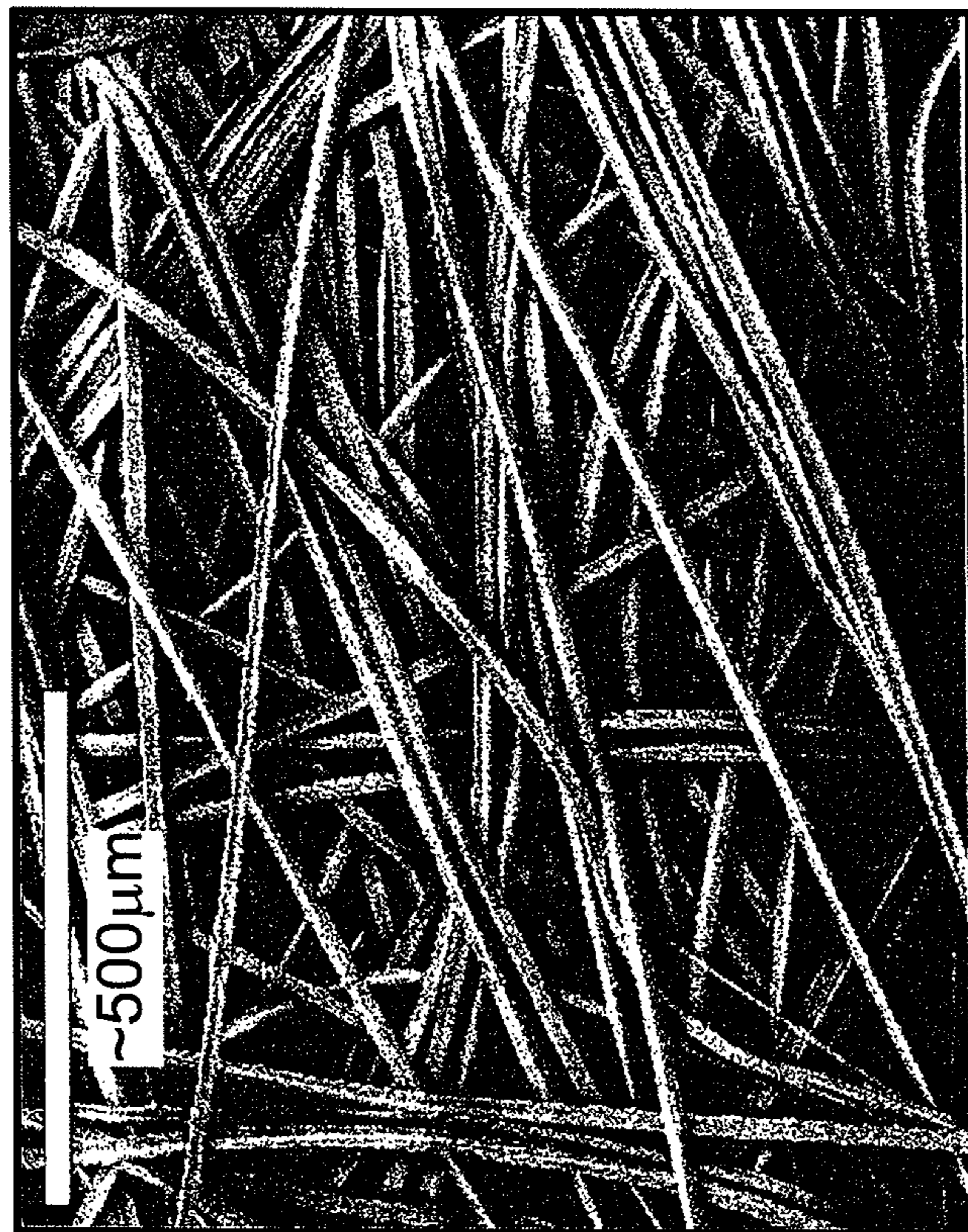
Thermally Bonded 100 gsm
