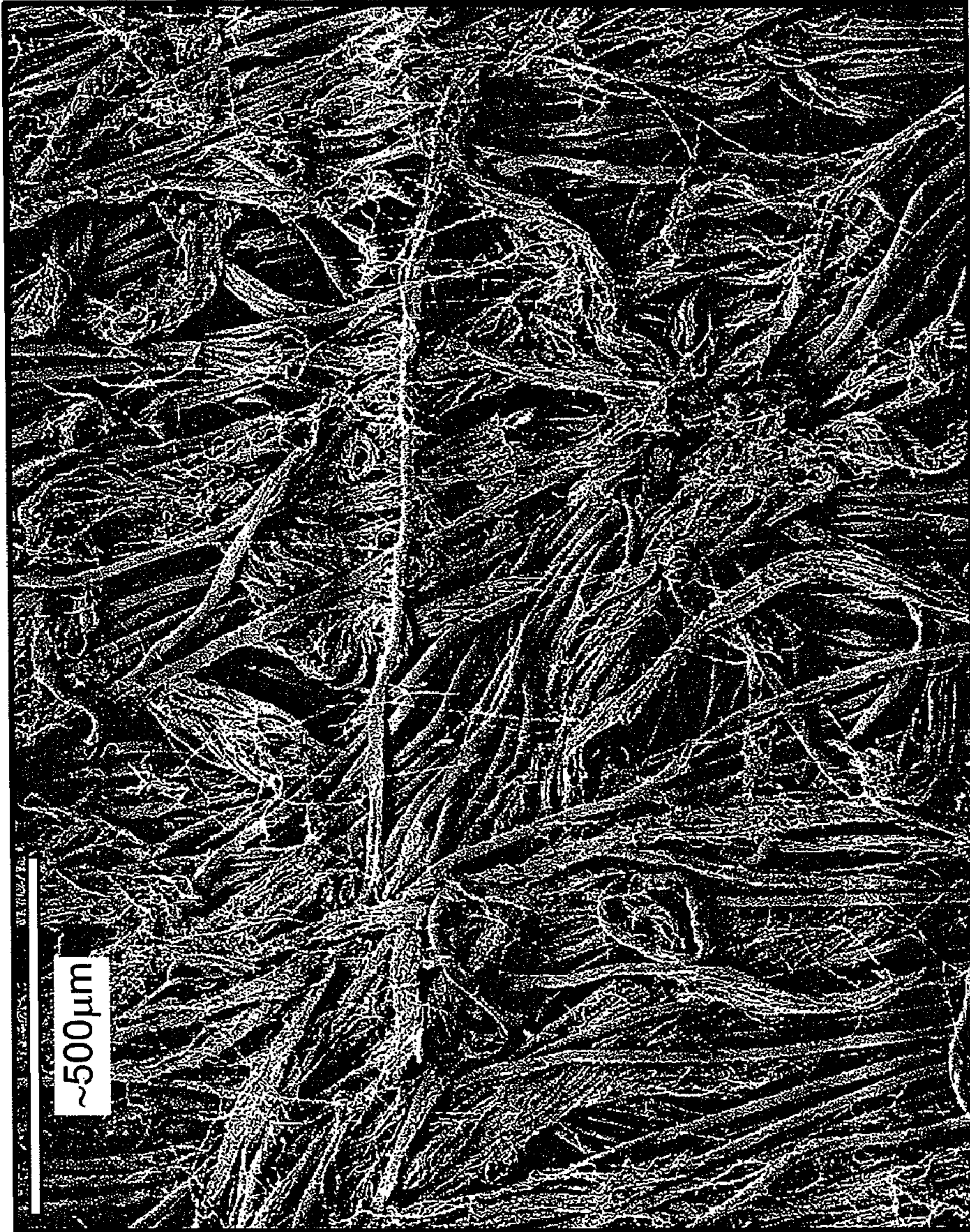
SEM Micrographs of Surface of an I-S Hydroentangled Spunbonded Fabric with Fibers Partially Separated
