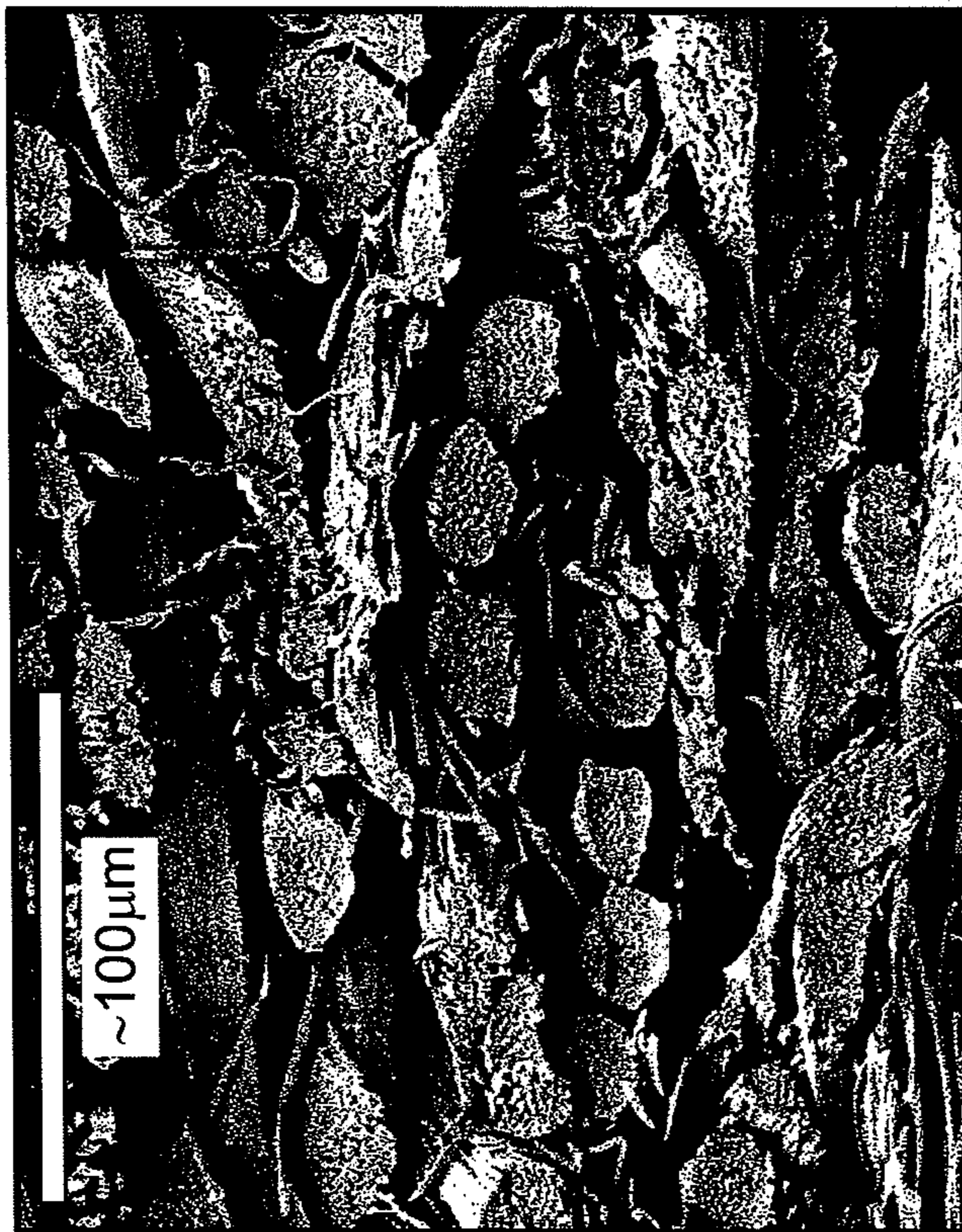
2 Hydro Passes + Point Bonded at 145 °C 180 - 200 gsm
