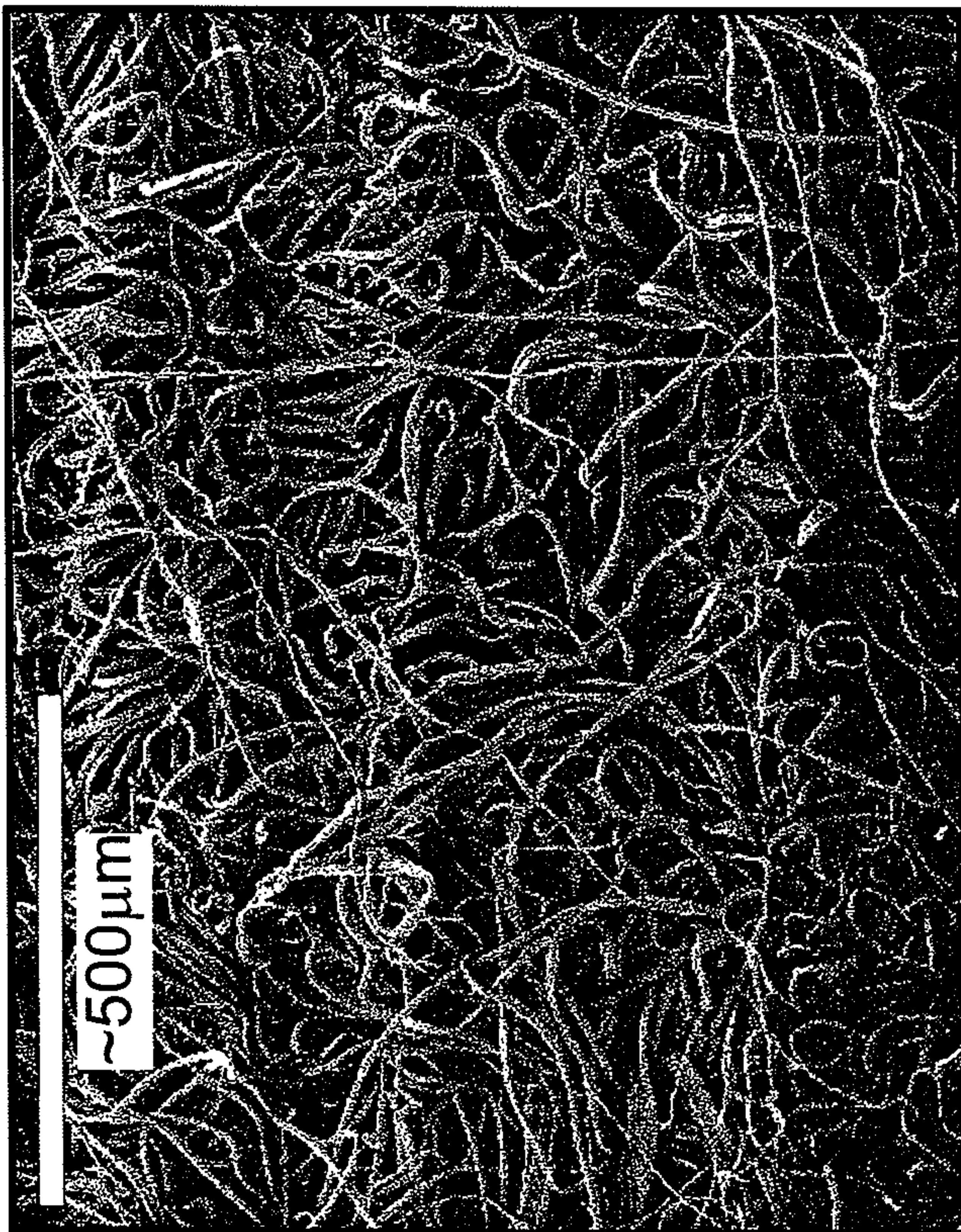
Hydroentangled and Fractured 100 gsm
