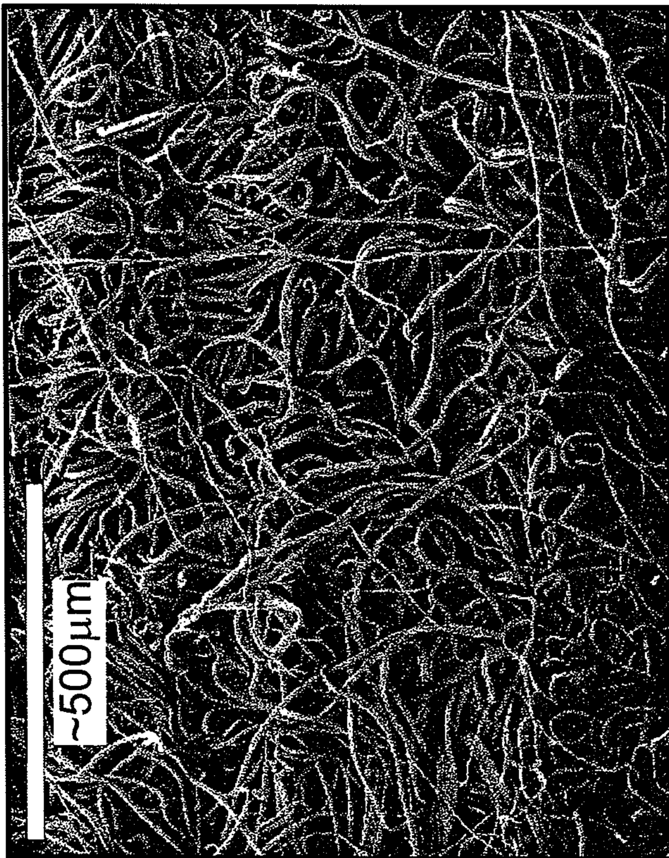
Hydroentangled and Fractured 100 gsm
