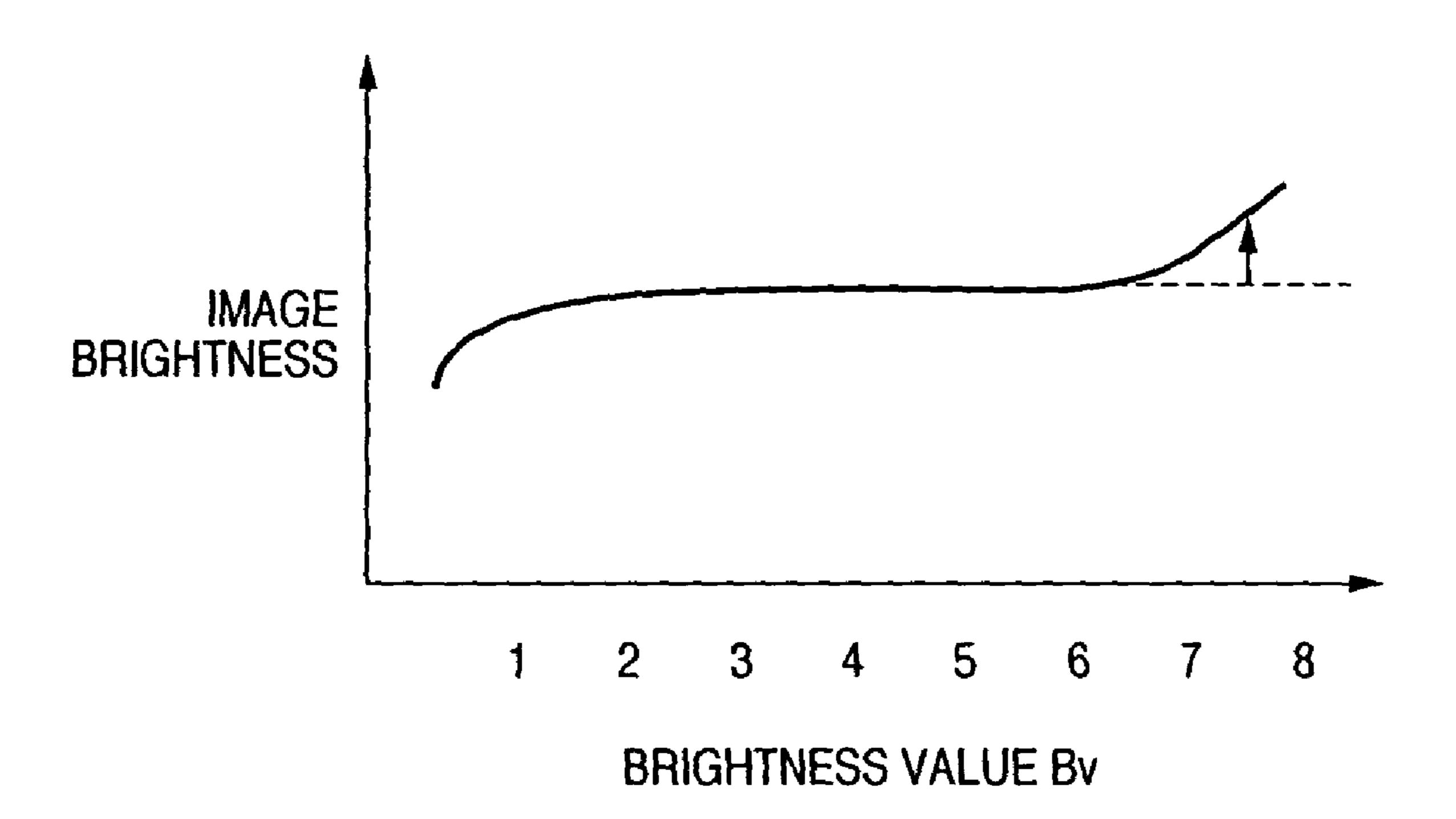
IMAGE SENSING APPARATUS, IMAGE SENSING METHOD, RECORDING MEDIUM, AND PROGRAM FOR CONTROLLING EXPOSURE BY CORRECTING A BRIGHTNESS VALUE WHEN AN OPTICAL FILTER IS MANUALLY INSERTED
