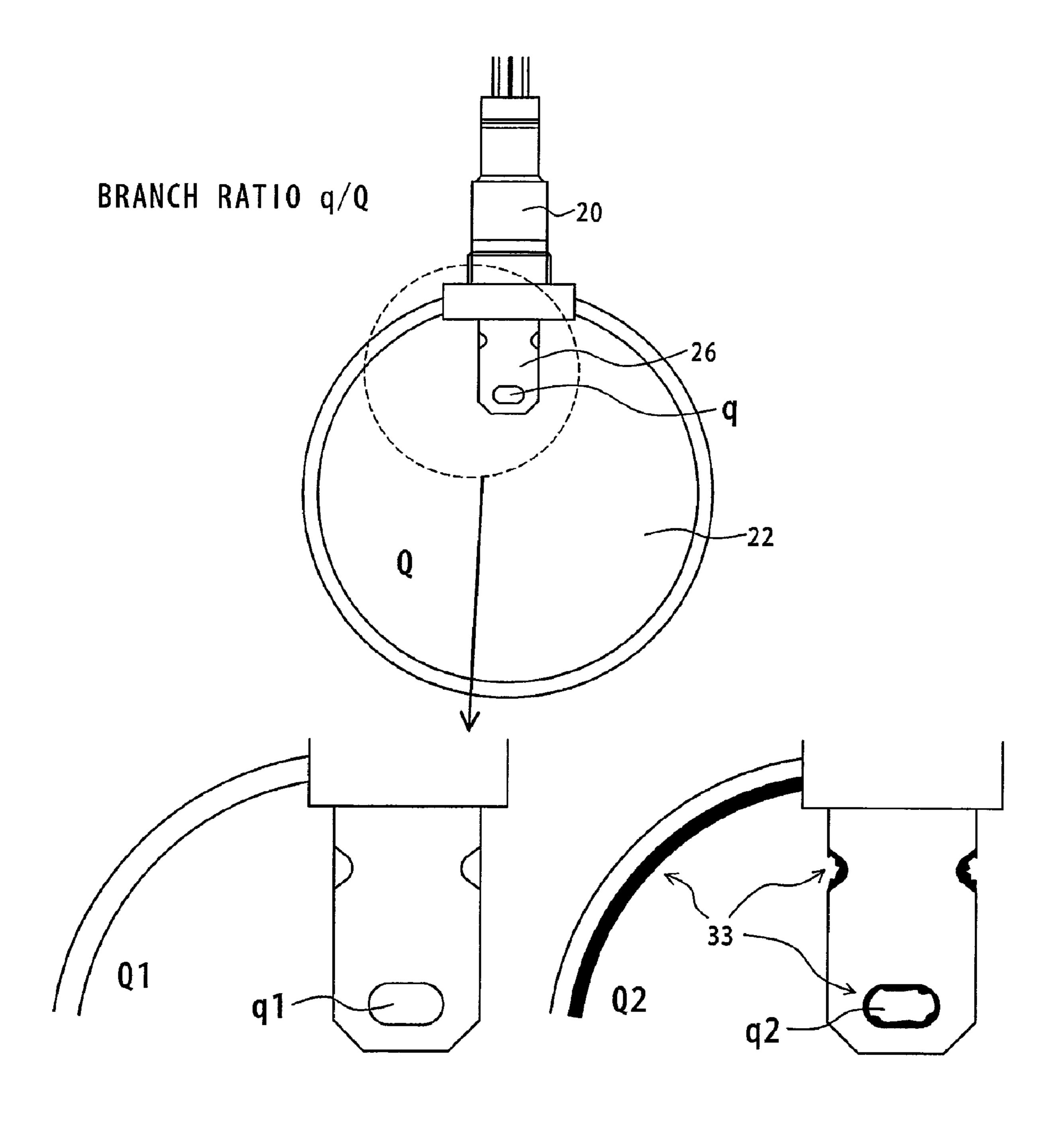
$Q_2/Q_1 \gg q_2/q_1$  BRANCH RATIO  $q_1/Q_1 <$  BRANCH RATIO  $q_2/Q_2$
