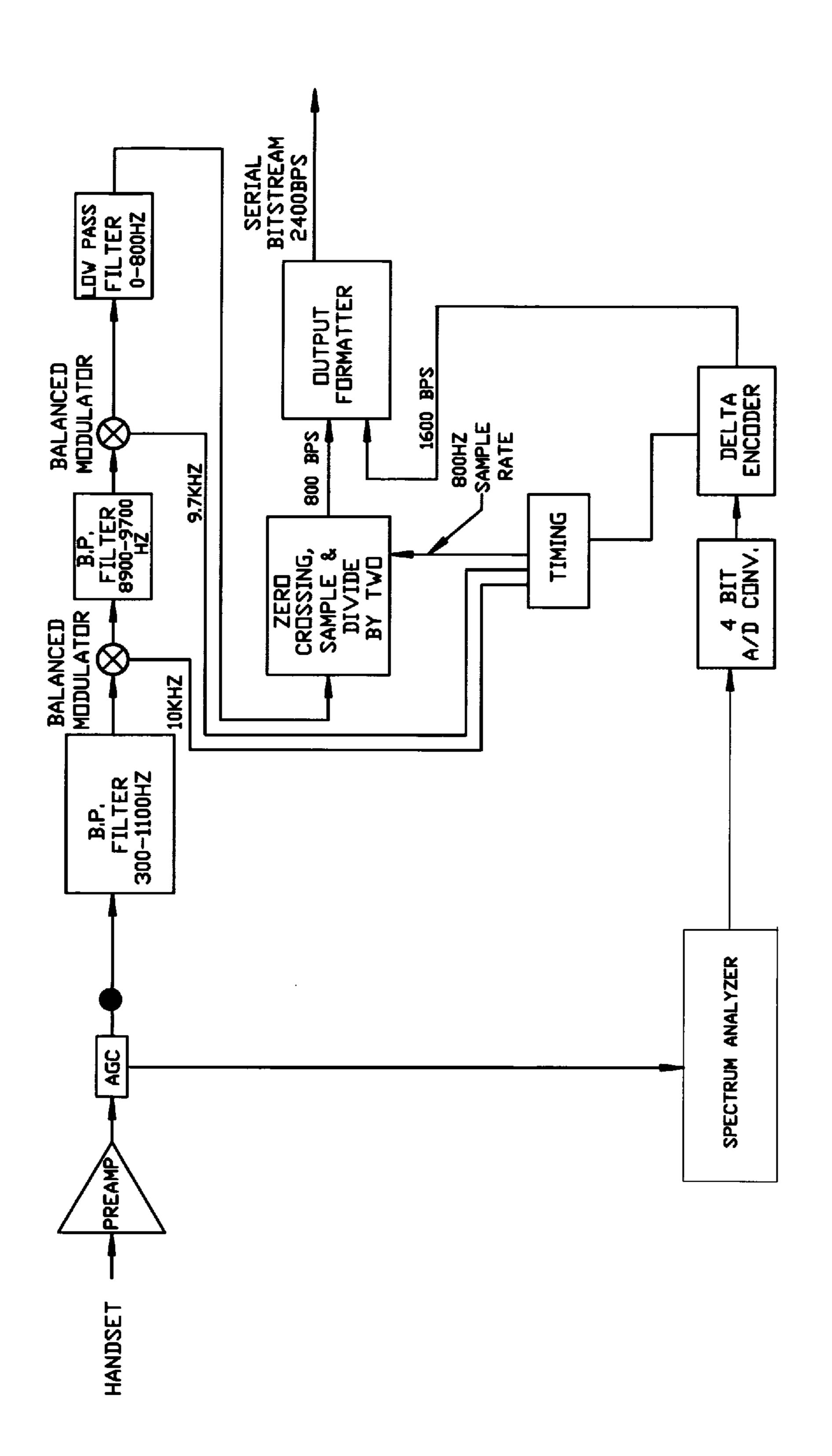
2400 BITS PER SECOND VOCODER TRANSMITTER
