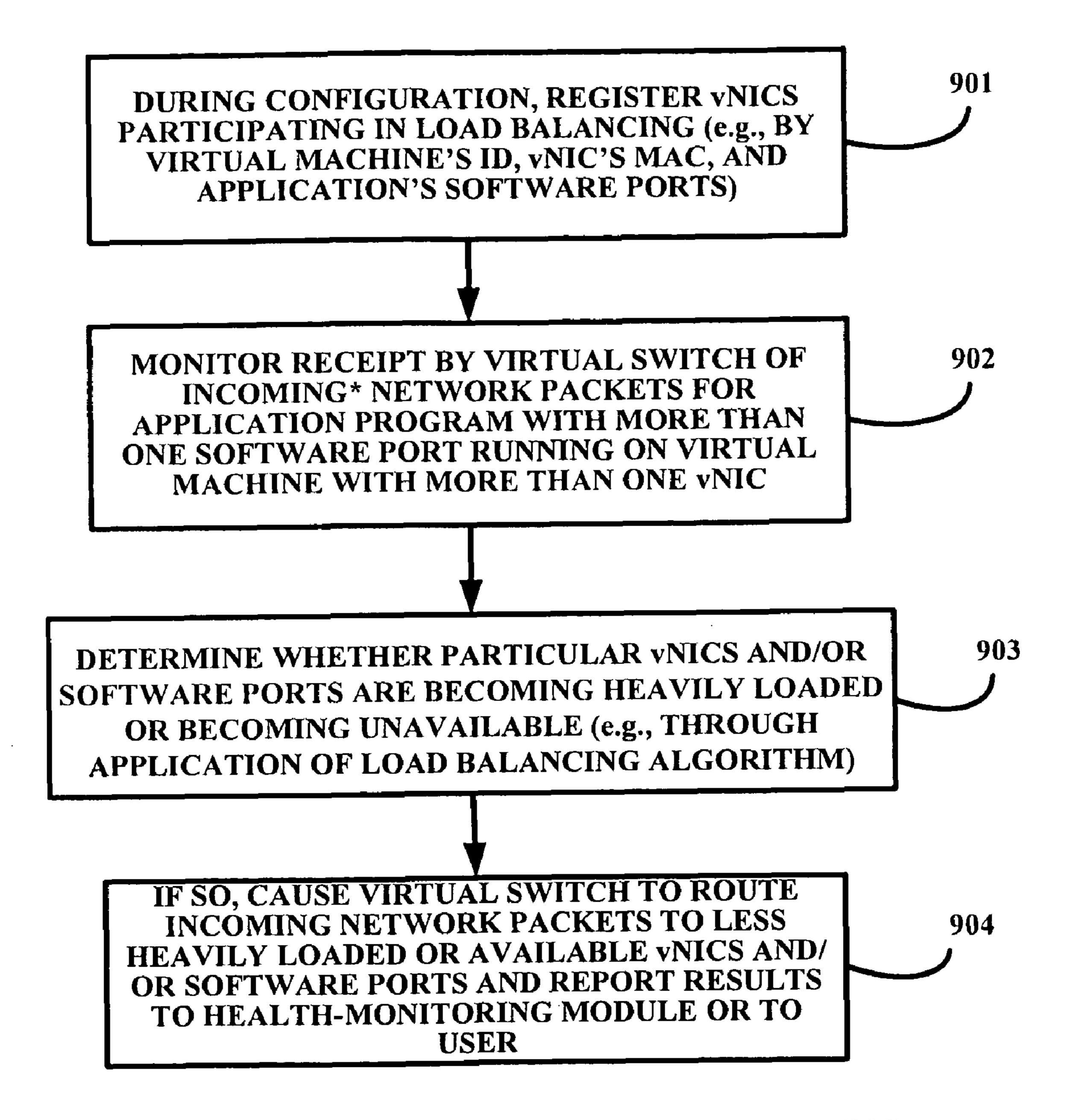
\*PROCESS WORKS EQUALLY WELL FOR OUTGOING NETWORK PACKETS FROM APPLICATION PROGRAM'S SOFTWARE PORTS
