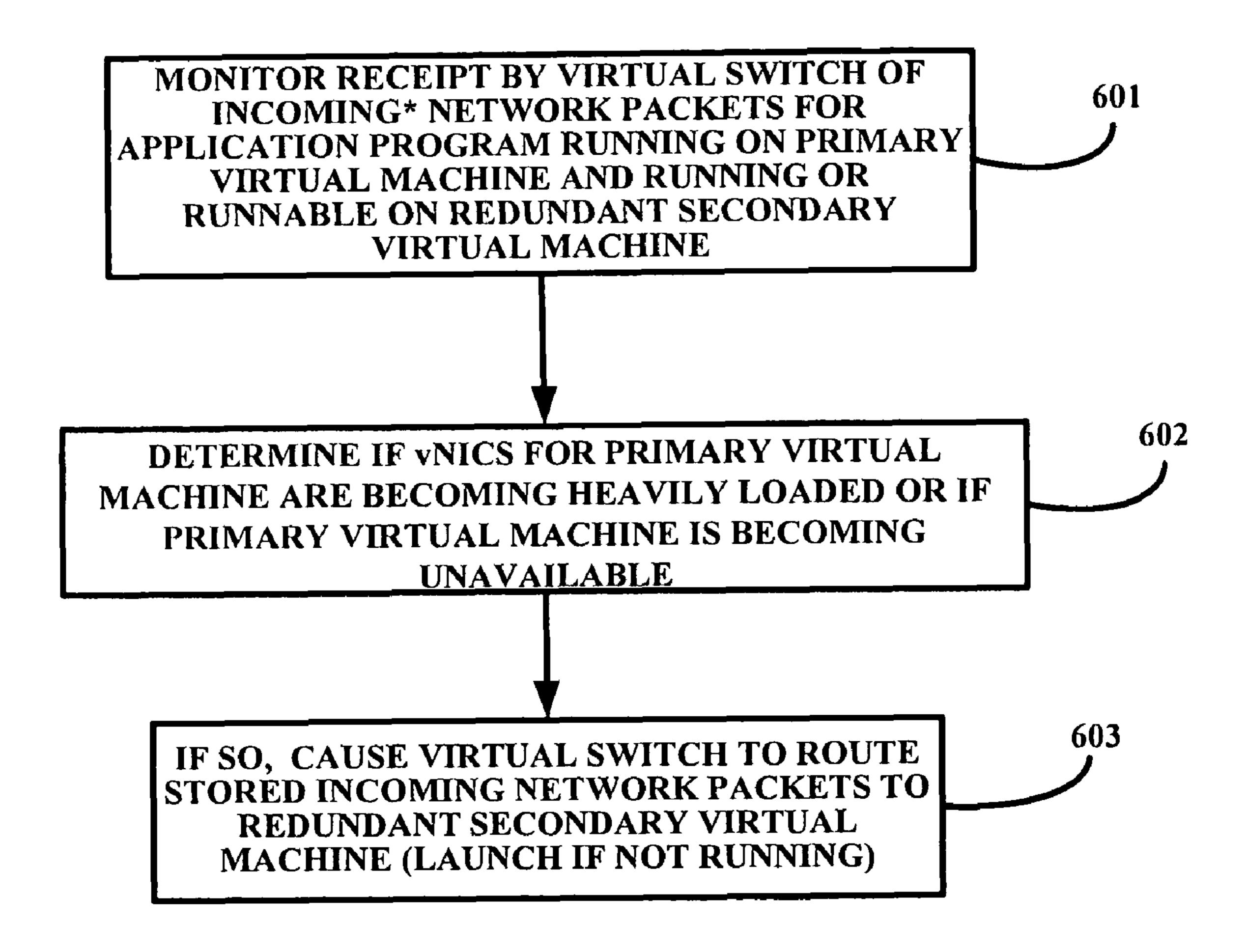
\*PROCESS WORKS EQUALLY WELL FOR OUTGOING NETWORK PACKETS FROM APPLICATION PROGRAM
