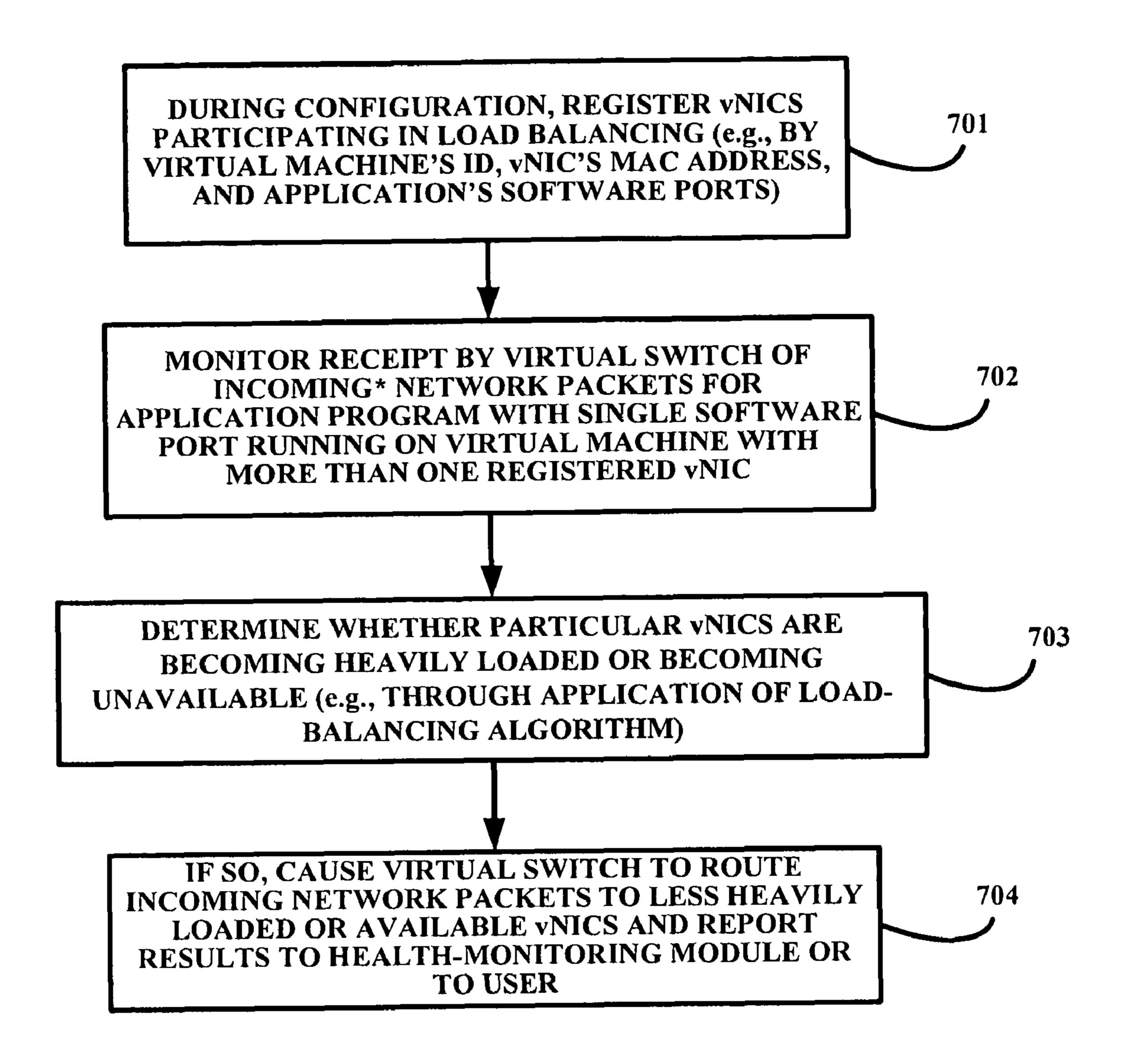
\*PROCESS WORKS EQUALLY WELL FOR OUTGOING NETWORK PACKETS FROM APPLICATION PROGRAM'S SOFTWARE PORT
