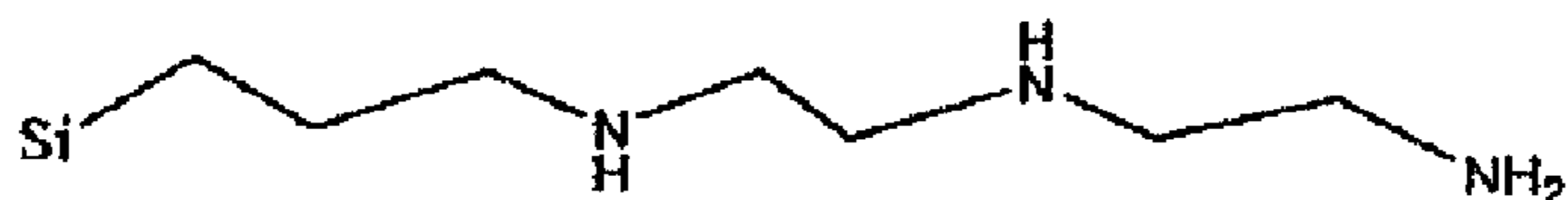
DPS: (3-diethylenetriamino)propyl-functionalized silica
