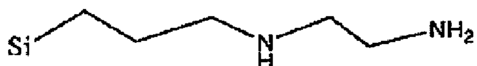
EPS: (3-ethylenediamino)propyl-functionalized silica
