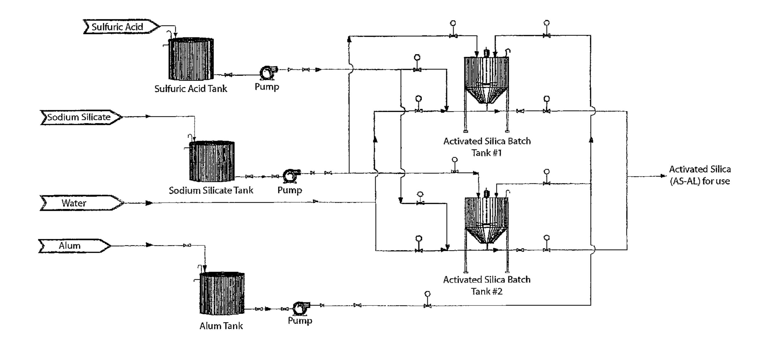
Figure 1. Activated Silica Preparation Diagram
